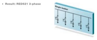
8 Feeder and 1 bus coupler, double busbar; decentral or central arrangement, busbar protection, breaker failure protection, busbar replica software, isolator supervision, event recorder with 1000 events, disturbance recorder, time synchronization, IEC 870-5-103 communication
