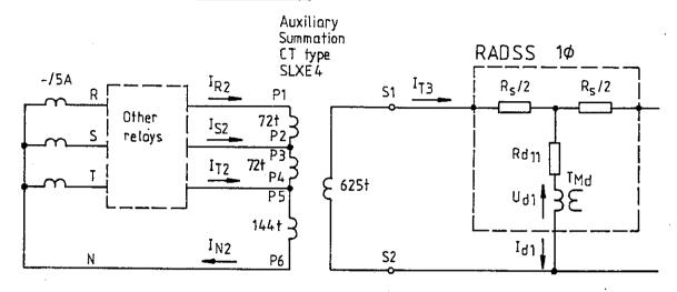
The minimum relay operating current is given by  $I_{T3} = I_{d1min}$
