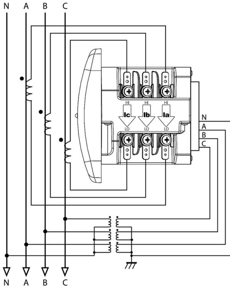
FIGURE 3-11: 4-Wire Wye with 3 PTs and 3 CTs, 3 Element
