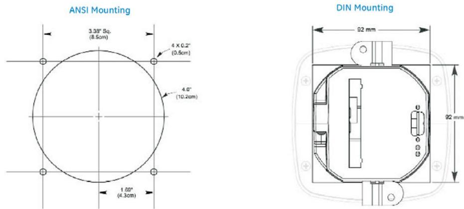
FIGURE 3-2: ANSI and DIN Mounting Panel Cutouts
