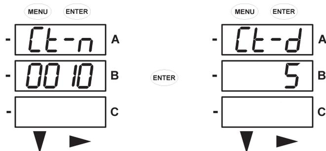
The **ct-d** value is preset to a 1 or 5 A at the factory and cannot be changed.
