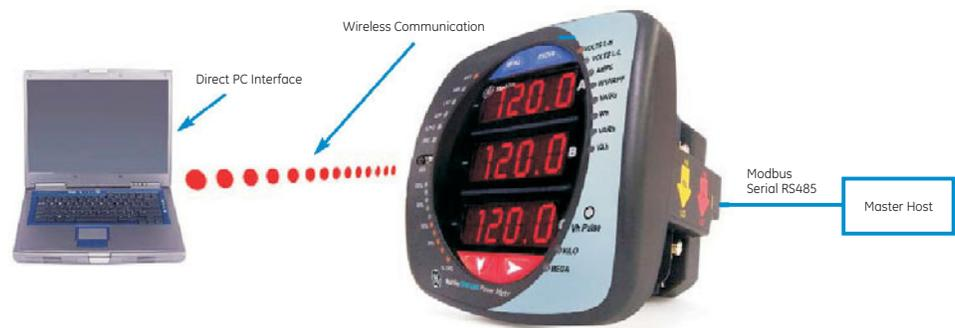
**FIGURE 3–15: Simultaneous Dual Communications Paths**
