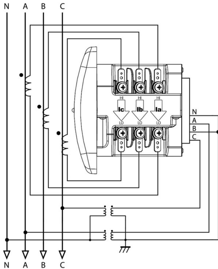
FIGURE 3-12: 4-Wire Wye with 2 PTs and 3 CTs, 2.5 Element
