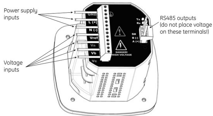
FIGURE 3-8: Voltage Connection
