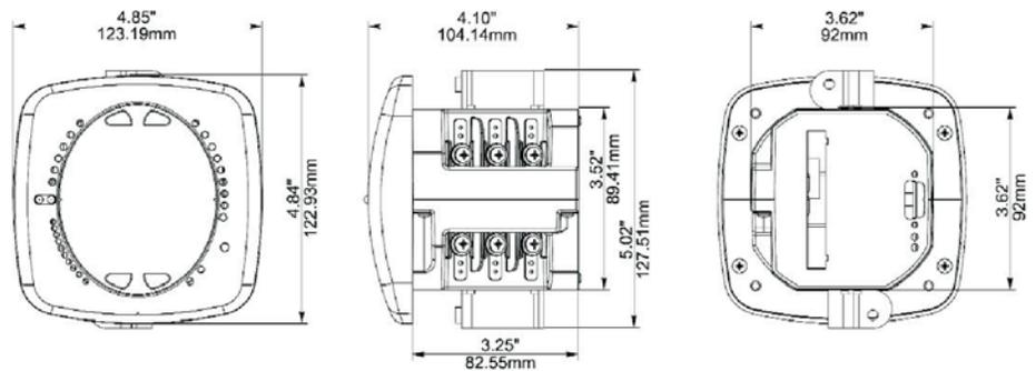
FIGURE 3-1: Bezel, Side, and Back Dimensions
