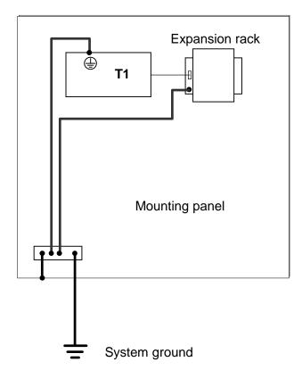
In case of the expansion rack is connected to the T1/T1S, the rack mounting screw is used for this purpose.
