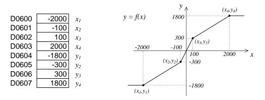
The FG instruction interpolators f(x) value for x based on the *n* parameters of  $(x_i, y_i)$ . For example, if XW04 is 1500 (x = 1500), the result 1405 (f(x) = 1405) is stored in D0100.
