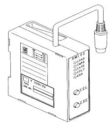
The program storage module (RM102) is an external memory for storing the T1/T1S program. By using the RM102, program saving from the T1/T1S to the RM102, and program loading from the RM102 to the T1/T1S can be done without need of a programmer. Because the RM102 has an EEPROM, maintenance-free program storage and quick saving/loading are available.
