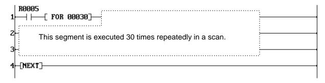
When R005 is ON, the program segment between FOR and NEXT is executed 30 times in a scan.
