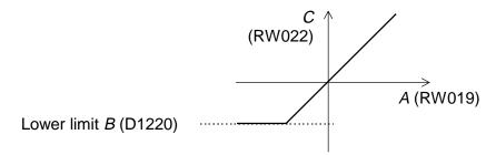
When RW019 is -1000 and D1220 is -1800, -1000 is stored in RW022 and R0041 is OFF. When RW019 is 800 and D1220 is 1200, the limit value 1200 is stored in RW022 and R0041 is ON.
