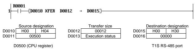
When R0001 is ON, one set of message (ended by the trailing code) stored in the range of D0500 to D0511 (12 words) is transmitted through the RS-485 port.
