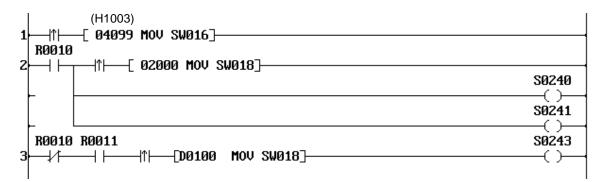
In this example, 4099 (H1003) is set in SW16. As a result, the single phase up-counter (channel 1 only) is selected.
