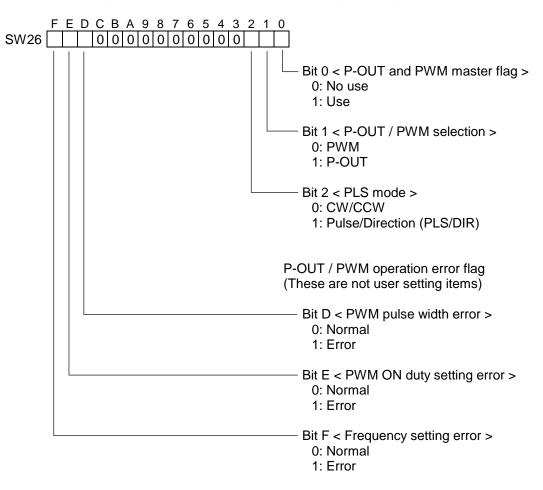
Note) In the explanation below, P-OUT means the pulse output function.
