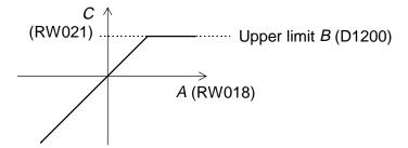
When RW018 is 3000 and D1200 is 4000, 3000 is stored in RW021 and R0040 is OFF. When RW018 is 4500 and D1200 is 4000, the limit value 4000 is stored in RW021 and R0040 is ON.
