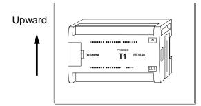
Mount the T1 on a vertical panel. All other mounting positions are not acceptable.
