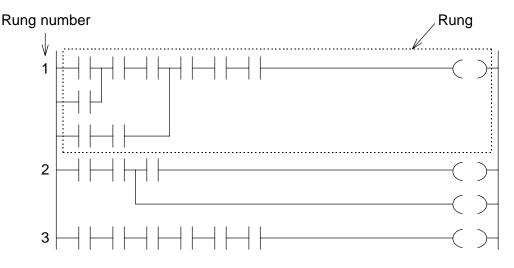
The rung numbers are a series of numbers (decimal number) starting from 1, and cannot be skipped. There is no limit to the number of rungs.
