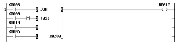
9 devices starting with R200 (R200 to R208) is specified as a shift register. When R010 is OFF, the data of the shift register is reset to 0. (R200 to R208 are reset to OFF) The carry flag (CF = S050) is also reset to OFF.
