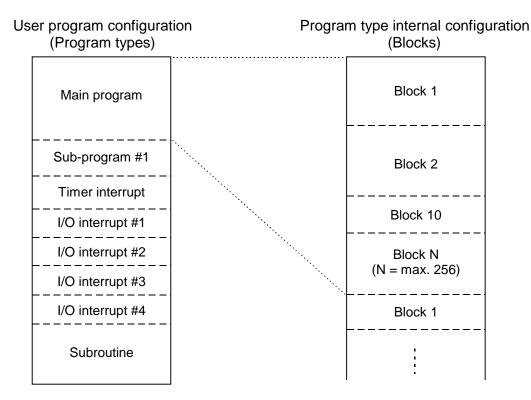
In the user program, the main program is the core. The scan operation explained in section 5.3 is for the main program. The operation of other program types are explained in the following sections.
