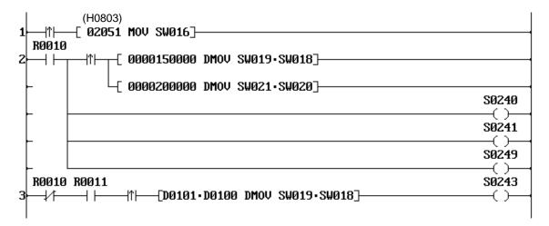
In this example, 2051 (H0803) is set in SW16. As a result, the quadrature bi-pulse counter is selected.
