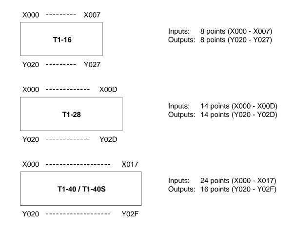
Any operation for the I/O allocation are not required if only the T1/T1S basic unit is used.
