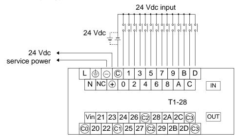
Note) The 24 Vdc service power output is not provided on the DC power supply type.
