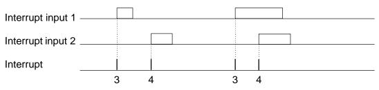
The above operation example is the case of rising edge setting for both inputs.
