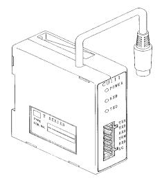
The T1/T1S's RS-232C programmer port supports the computer link function. When two or more T1/T1Ss are connected with a master computer, the multi-drop adapter (CU111) can be used. (One-to-N configuration) The CU111 is an RS-232C/RS-485 converter specially designed for the T1/T1S's programmer port.
