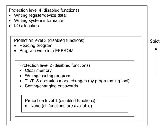
When the level 1, 2 and 3 passwords are registered, the T1/T1S will be started as protection level 4. In this state, for example, entering the level 2 password changes the protection level to 2.
