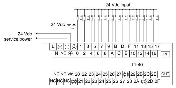
Note) The 24 Vdc service power output is not provided on the DC power supply type.
