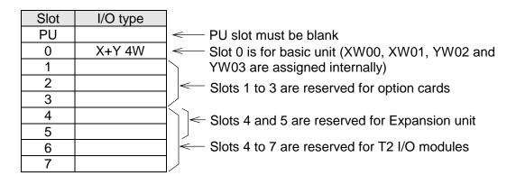
The T1/T1S operating system automatically sets the I/O type 'X+Y 4W' on the slot 0 position when the memory clear is executed for the T1/T1S.
