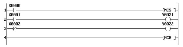
When X000 is OFF, Y021 and Y022 are turned OFF regardless of the states of X001 and X002.
