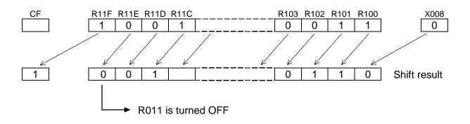
The figure below shows an operation example. (When X009 is changed from OFF to ON)
