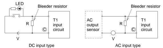
Select a bleeder resistor according to the following criteria:
