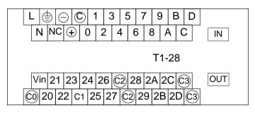
T1-MAR28 ... AC power supply, AC input type
