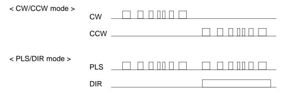
In the both modes, pulse output is enabled when the pulse enable flag is ON. While the pulse enable flag is ON, the pulse frequency can be changed by changing the frequency setting value. However, the pulse direction (the sign of the frequency setting) cannot be changed when the pulse enable flag is ON.
