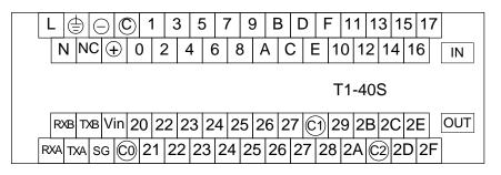
T1-MAR40S ... AC power supply, AC input type
