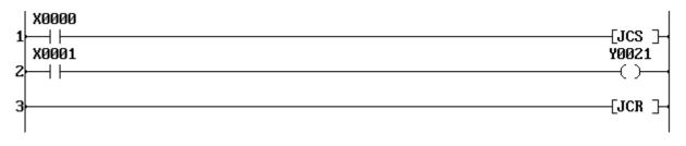
When X000 is ON, the rung 2 circuit is skipped, therefore Y021 is not changed its state regardless of the X001 state. When X000 is OFF, Y021 is controlled by the X001 state.
