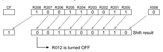
(When X00A is ON and X009 is changed from OFF to ON)
