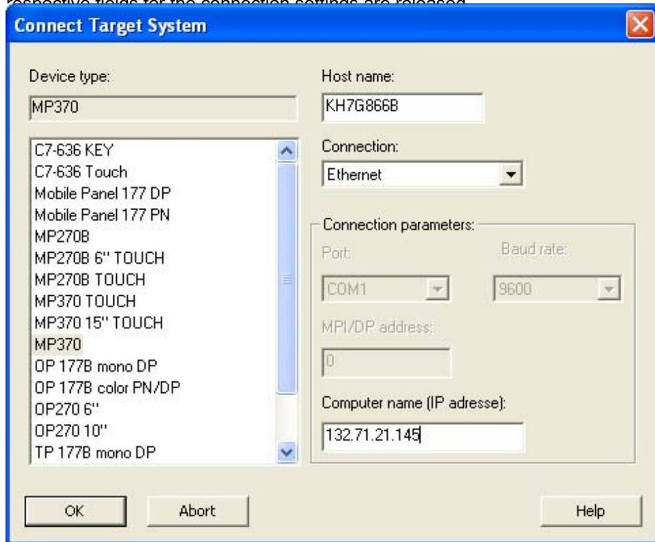
3. Select the required connection parameters and then click on "OK". A connection with the HMI device is created. The connected HMI device is displayed in the left window of the Automation License Manager.
