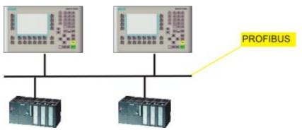
Such systems are deployed, for example, in a production line to operate the plant from several points.
