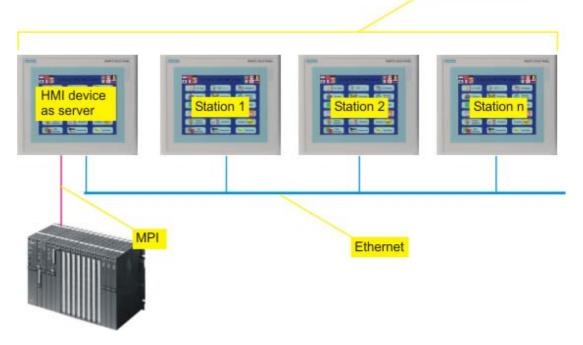
Only one HMI device contains the configuration data and functions as the server. The server can be controlled from the other operator devices. All the HMI devices display the same screens.
