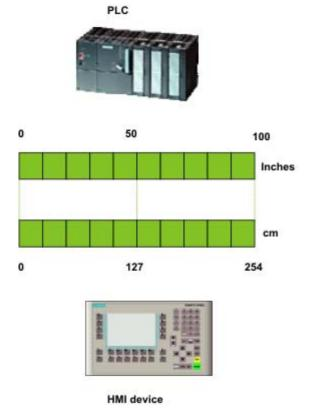
As soon as data from the HMI device is written to an external tag, it will be automatically mapped to the value range of the PLC. As soon as data from the HMI device is read from the external tag, a corresponding transformation will be performed in the other direction.
