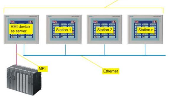
Only one HMI device contains the configuration data and functions as the server. The server can be controlled from the other operator devices. All the HMI devices display the same screens.
