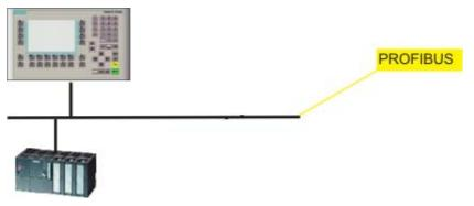
Single-user systems are generally used near production, but can also be deployed to operate and monitor independent part processes or system sections.
