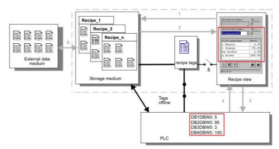
A reading device connected to the PLC reads a bar code on the work piece to be processed. The recipe data record names correspond to the respective bar code names. This will enable the PLC to load the necessary recipe data record from the storage medium of the HMI device. The recipe data record is displayed for inspection. Changes are transferred immediately to the PLC.
