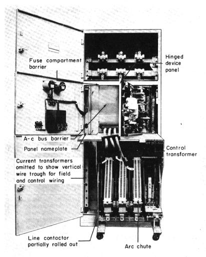
Fig. 9. Free entrance to controller gained by rolling out IC2812 contactor
