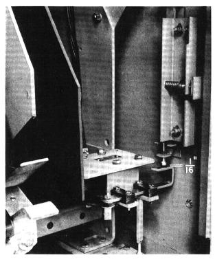
Fig. 12. Contactor mechanical interlock adjustment
