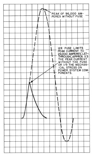
Fig. 3. Current-limiting action of Type EJ-2 fuse
