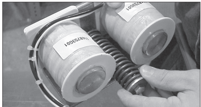
Fig. 20 Unscrew the return spring assembly
