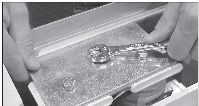
Fig. 19 Remove the locknut securing the return spring bolt
