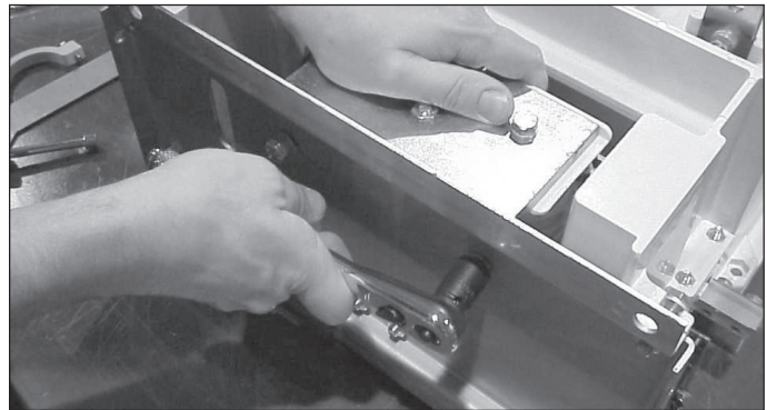
Fig. 18 Remove the coil mounting angle
