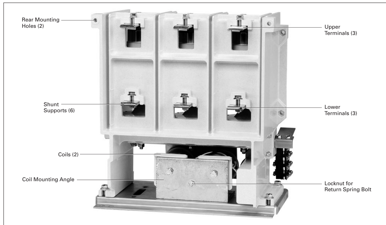
Figure 2. SL Rear View Major Components
