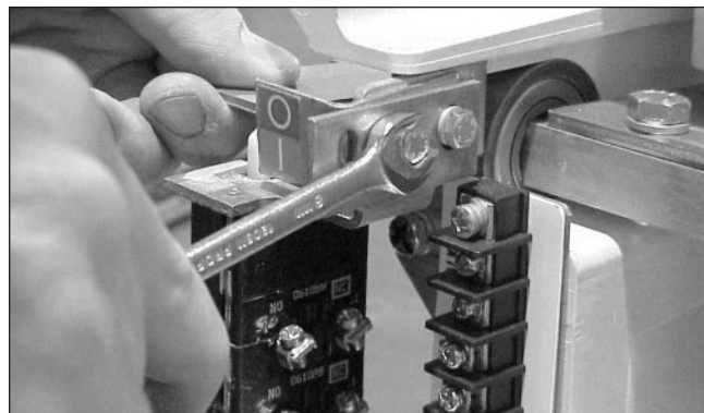
Figure 27. Remove the Two Mounting Screws Securing the Contact Assembly to Bearing Retainer
