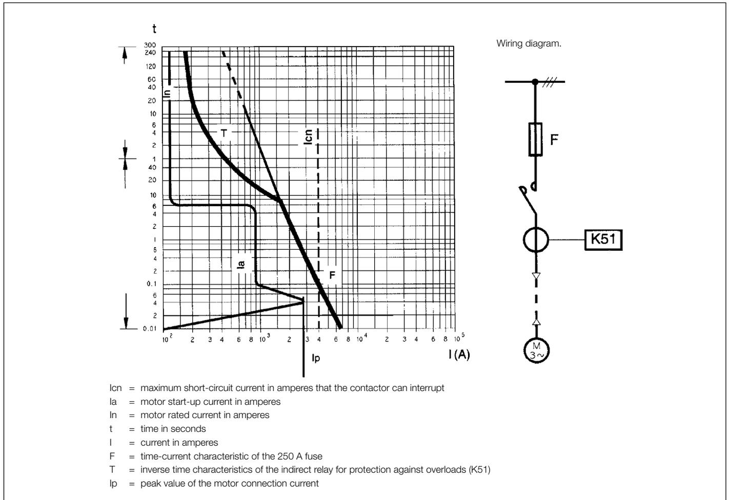
Fig. D - Graph showing the coordination between 250 A fuse and relay with inverse time delay trip.
