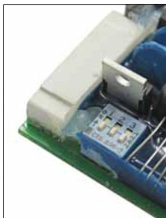
First of its type, the V-Contact VSC contactor is fitted with an undervoltage function with selectable delays of 0; 0,5; 1; 2; 3; 4; 5 s.
