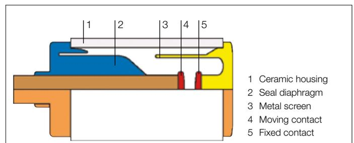
Schematic cross-section of the vacuum interrupter.
