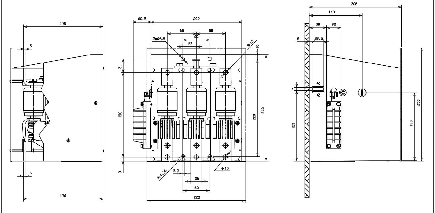
VSC 3 fixed contactor (95 mm connection centre distance)
