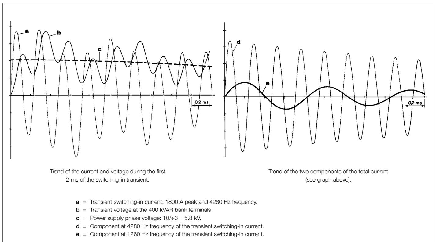
Fig. B - Example of a current transient during connection of a capacitor bank with another one already supplied with voltage.
