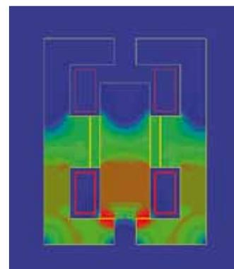
Fig. C - Magnetic circuit in the open position.
