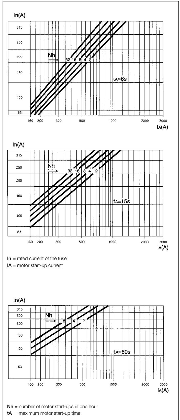
Fig. A - Fuse selection curves for motor start-up. ABB CMF type fuses.
