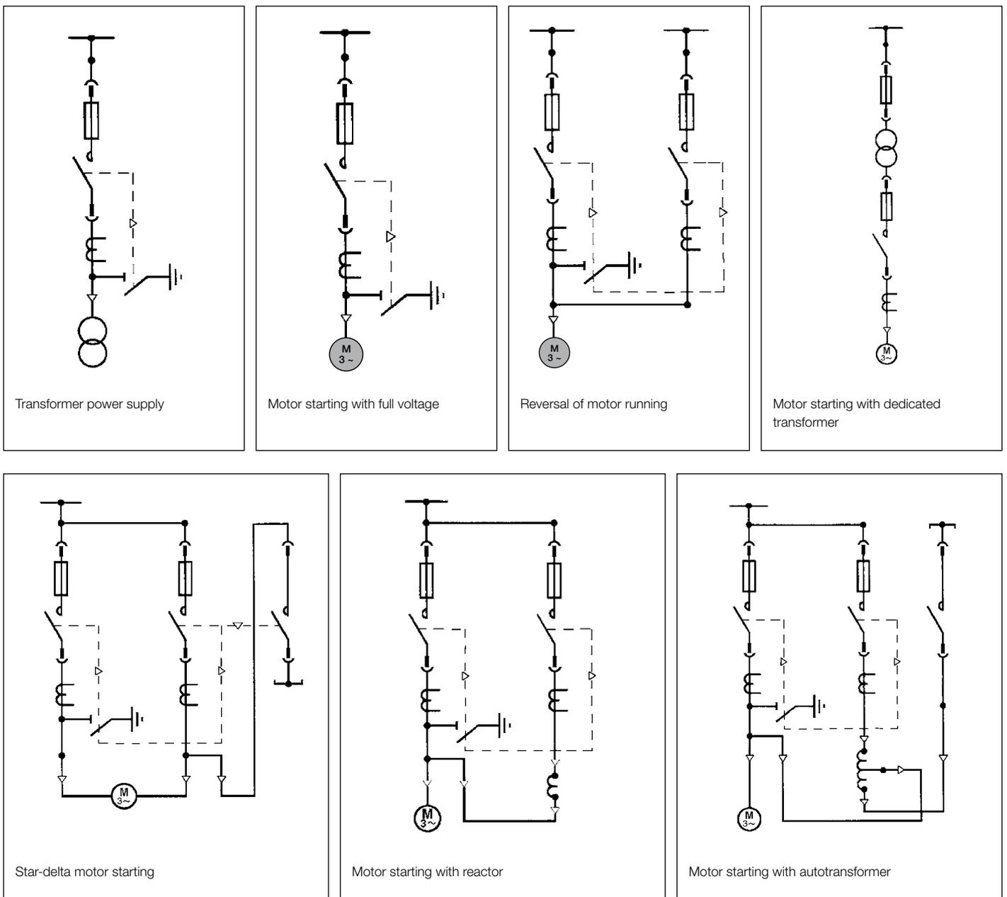
Fig. E - Typical diagrams of transformer power supply and motor starting
