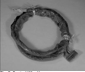
Fig. 7 Control Wire Harness
