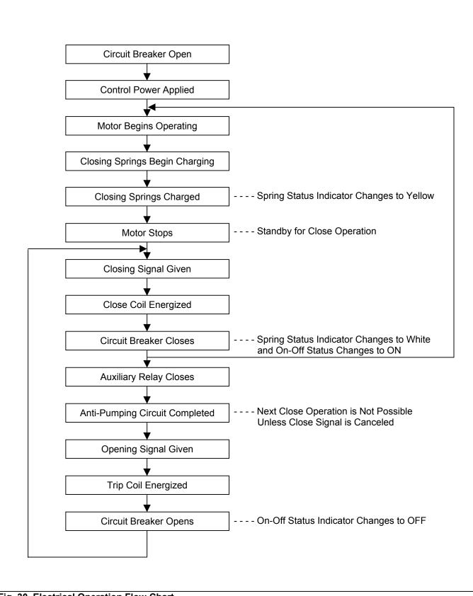
Fig. 30 Electrical Operation Flow Chart
