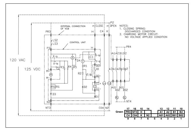
Fig. 31 125 VDC Control Circuit Schematic
