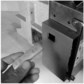
Fig. 29 Removing Plug From UV Trip Device
