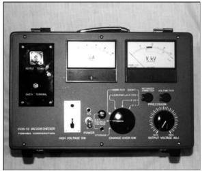
Fig. 33 Toshiba Portable Vacuum Checker
