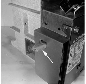
Fig. 28 Plug Installed in UV Trip Device
