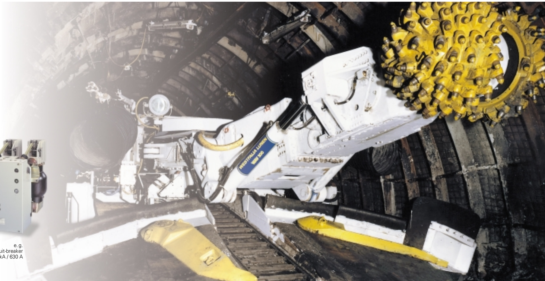
Mobile selective-cut road driving machine for underground mining type WAV 300 (photo Westfalia Lünen)
