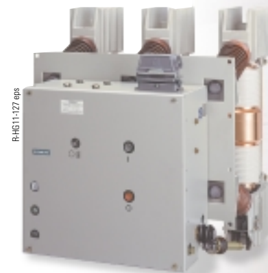
e. g. 3AH4 frequent-operation circuit-breaker 24 kV / 40 kA / 2500 A (partitions not shown)
