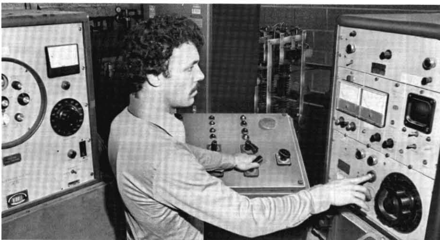
Final production tests are made on each circuit breaker including Corona and High-Pot tests to industry standards.
