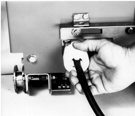
FIGURE 3.3.3 INSERT REMOTE OPERATING STATION PLUG
