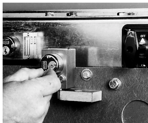
FIGURE 3.4.24 INSERT KEY KD IN KEY LOCK K5 AND ROTATE
