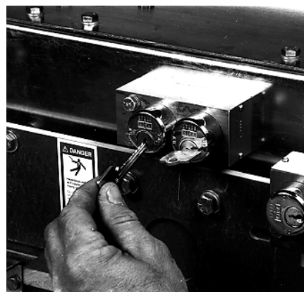
FIGURE 3.5.22 REMOVE KEY KC FROM KEY LOCK K2
