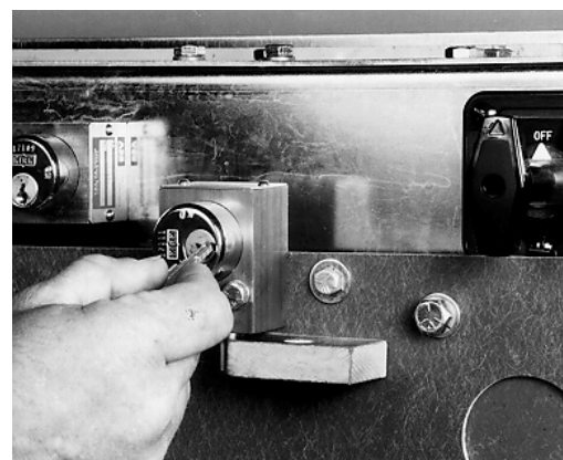
FIGURE 3.5.10 REMOVE KEY KD FROM KEY LOCK K4
