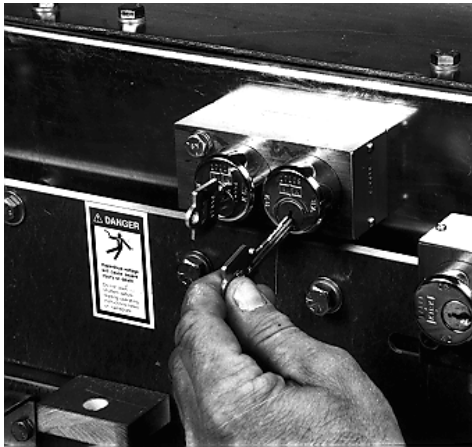
FIGURE 3.2.3 INSERT KEY KB IN KEY LOCK K2 AND ROTATE KEY KC
