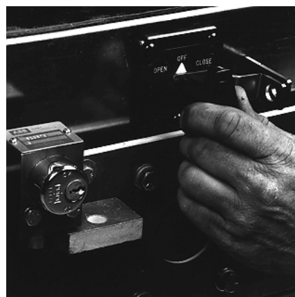
FIGURE 3.5.6 TURN SELECTOR SWITCH TO "OFF" POSITION
