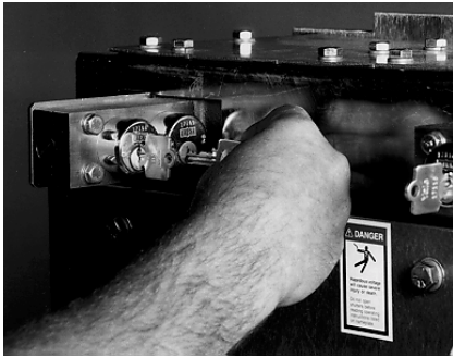
FIGURE 3.3.1 INSERT KEY KB IN KEY LOCK K1 AND ROTATE KEY KU
