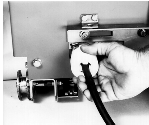
FIGURE 3.2.16 INSERT REMOTE OPERATING STATION PLUG
