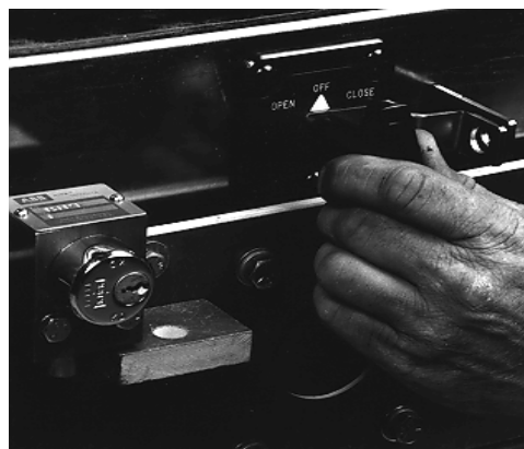
FIGURE 3.5.18 TURN SELECTOR SWITCH TO "OFF" POSITION
