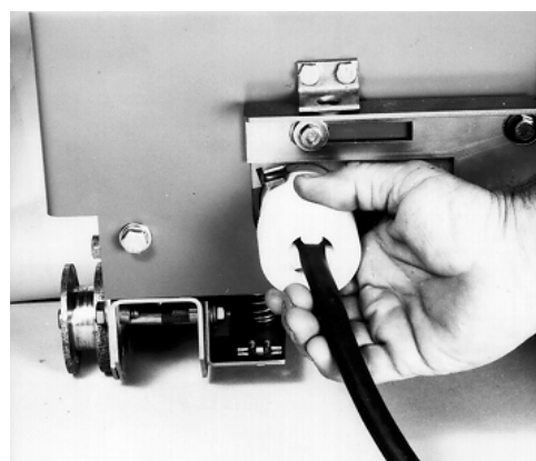
FIGURE 3.4.34 REMOVE REMOTE OPERATING STATION PLUG
