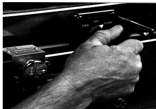
FIGURE 3.5.4 TURN SELECTOR SWITCH TO "CLOSE" POSITION
