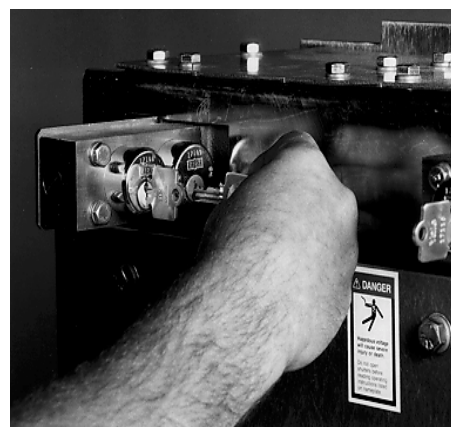
FIGURE 3.4.30 INSERT KEY KB IN KEY LOCK K1 AND ROTATE KEY KU
