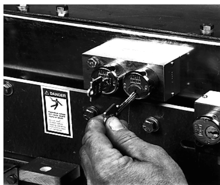
FIGURE 3.4.13 REMOVE KEY KB FROM KEY LOCK K2.
