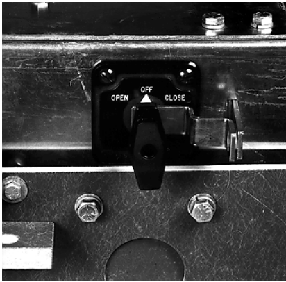
FIGURE 3.2.15 VERIFY THAT THE SELECTOR SWITCH IS IN THE "OFF" POSITION
