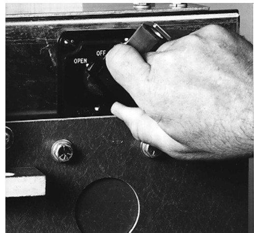
FIGURE 3.3.4 TURN SELECTOR SWITCH TO "OPEN" POSITION
