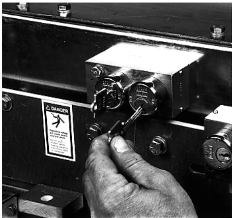
FIGURE 3.5.21 INSERT KEY KB IN KEY LOCK K2 AND ROTATE KEY KC
