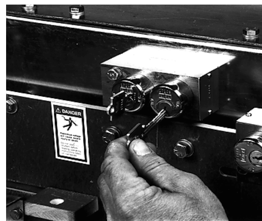
FIGURE 3.5.28 REMOVE KEY KB FROM KEY LOCK K2
