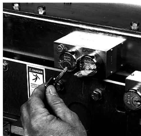
FIGURE 3.3.10 REMOVE KEY KC FROM KEY LOCK K2
