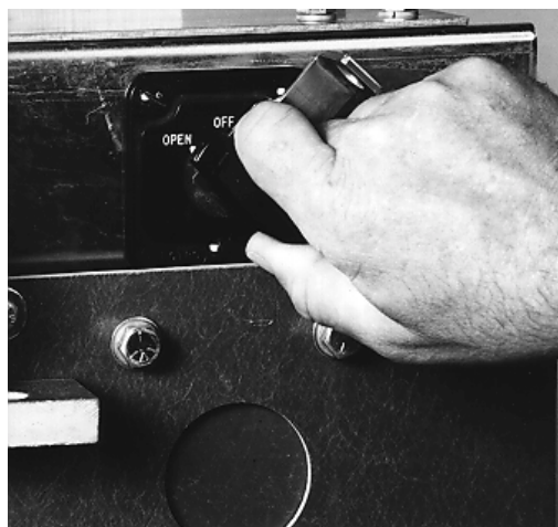
FIGURE 3.5.16 TURN SELECTOR SWITCH TO "OPEN" POSITION.
