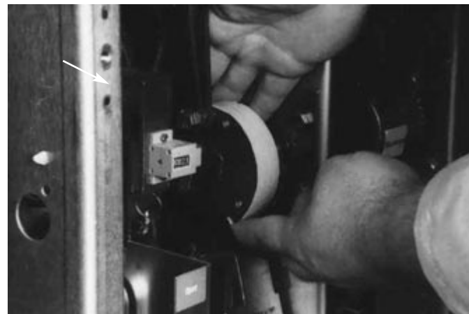
Figure 6-8 Attaching Tape Around to Back of Cam
