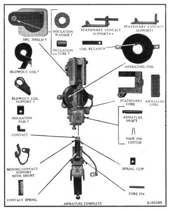
\*\* Used only on Contactors without blowout.
