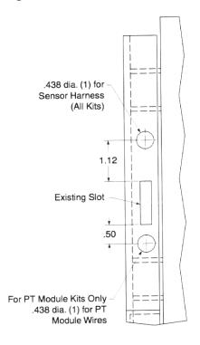
B. Cut and install the insulated tubing supplied on each PT Wire. Route the three (3) PT wires from the PT Module to the left rear of the Breaker, through the hole just drilled in Step 10-A, then down towards the Breaker Stabs.
