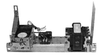
A. Mount the Breaker Mounted CPT to the CPT Mounting Plate as shown using the (2) .190-32 × .500" flat head screws, (2) .190-32 × .500" filister head screws, (6) flat washers, (4) lock washers, and (4) nuts supplied. Note the orientation of the CPT to the holes in the Mounting Plate. The CPT must be mounted in this orientation.
