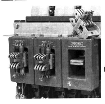
A. Remove the "E" clips and pins securing the Finger Clusters to the top Breaker Stabs. Remove the Finger Clusters. B. Apply Loc-Tite<sup>®</sup> 242 to the threads then secure the Sensors to the Mounting Angle using the (6) .250-20 × .500" bolts, (6) lock washers, and (6) flat washers supplied.
