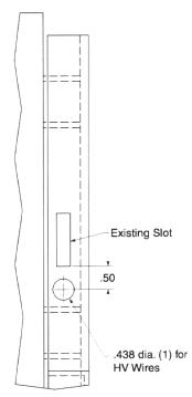
C. Route the HV Wires up through the Breaker, then through the hole just drilled towards the Phase 1 and 2, or 2 and 3 Top Breaker Stabs.
