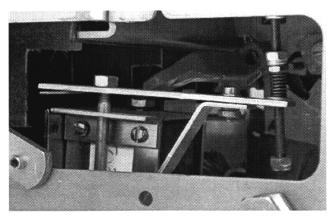
H. Connect the new Auxiliary Switch Drive Link to the left hand Auxiliary Switch (be sure to install it in the same orientation as original) using the (2) pins, (4) .250 flat washers, and (4) .06 × .88" cotter pins supplied.
