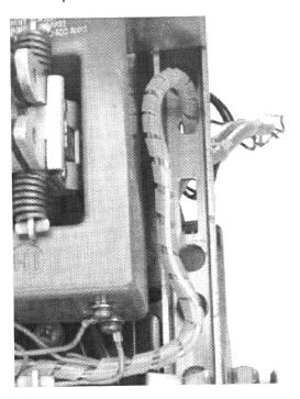
E. Connect the ring terminals of the Sensor Harness to the Sensors. Refer to Section 12 of the Retrofit Application Data, supplied with the Retrofit Kit, for detailed wiring specifications.
