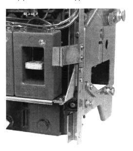
G. For Breakers equipped with a Secondary Contact Bracket, rotate the Secondary Contact Bracket, loosened in Step 2-A, to its original position. Secure it by reinstalling the original top screws and tightening the bottom screws.
