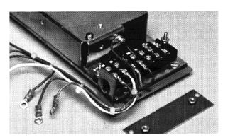
Note: The Glass Poly Insulation Plate that covers the 7-Point Terminal Block should not be reinstalled until the DTA Wires have been connected later in the Retrofit Process.
