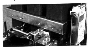
B. Align the Glass Poly Insulation Barrier with the existing studs then place it against the Arc Chute Retaining Bar. Secure the Insulation Barrier and the Arc Chute Retaining Bar, using the (2) flat washers, (2) lock washers, and (2) .250-20 nuts supplied. Note that the two (2) small holes on the Insulation Barrier must align with the holes in the Arc Chute Retaining Bar.
