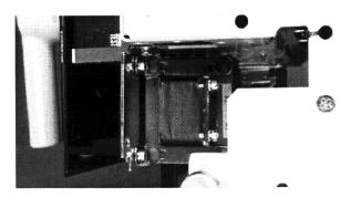
C. Strip .250" of insulation and attach a .138" ring terminal to each wire of the CPT Harness. Connect the wires to the X1 and X2 terminals of the CPT. D. Attach the HV Wires to the CPT terminals to achieve the required voltage. (See the following Table.)
