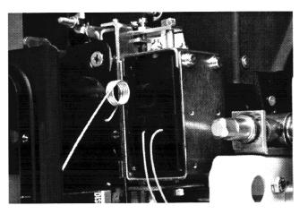
A. Drill and tap the two existing holes on the top of the right center Breaker Frame to accept .138-32 screws.
