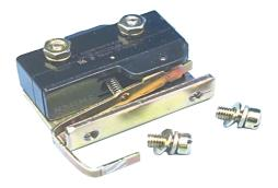
Align the Aux. Switch Assembly with the holes in the DTA Assembly. Secure the Aux. Switch Assembly to the DTA Assembly, as shown, using the (2) .190-32 x .375" screws, (2) flat washers, and (2) lock washers provided.
