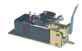
Insure that Aux. Switch moves to the "Closed" position when the DTA Reset Arm is moved towards the DTA.
