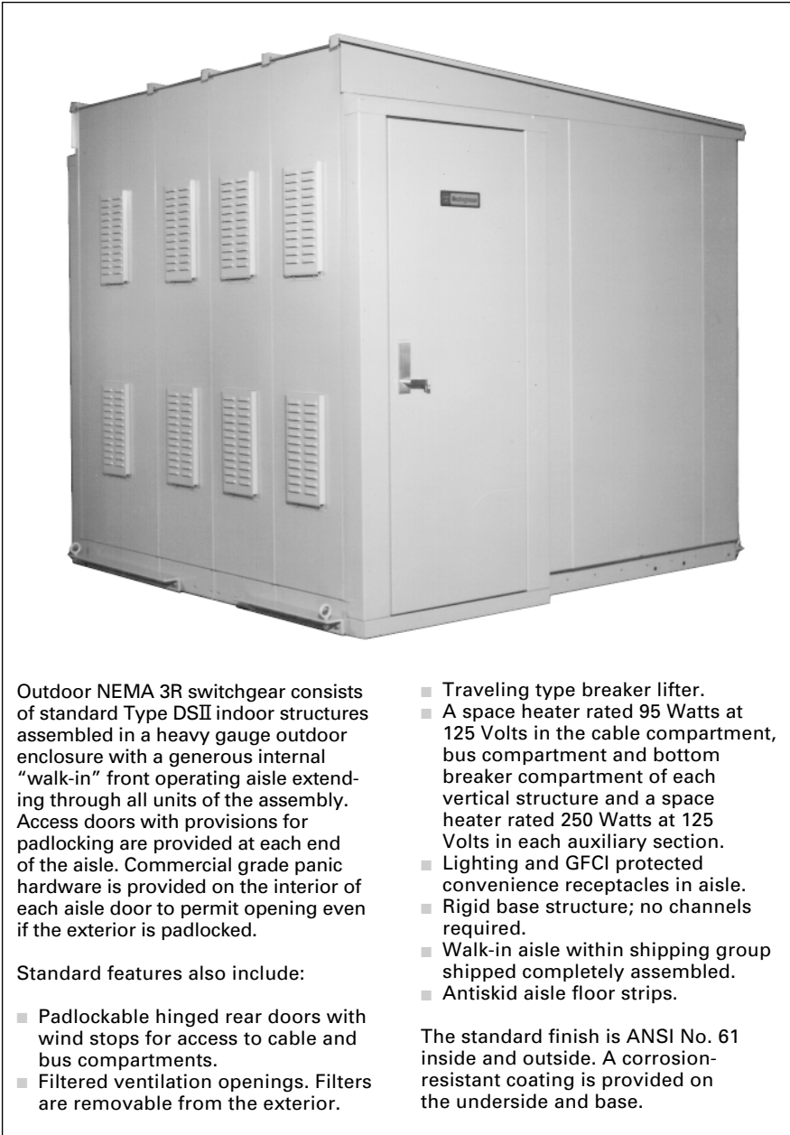
Outdoor Aisle Type Switchgear Enclosure
