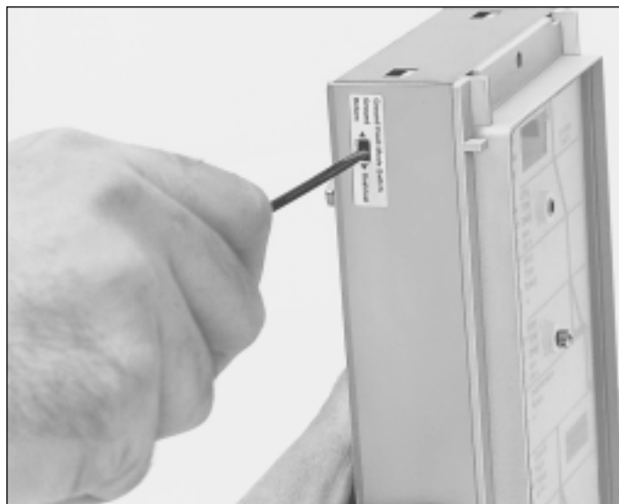
3. Set ground fault selection switch.
