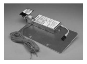
C. Align the Glass Poly Insulation Barrier with the holes in the back of the Aux. CT Module. Secure the Glass Poly Insulation Barrier to the Aux. CT Module, as shown, using the (2) .190-32 x .500" screws, (2) lock washers, and (2) flat washers supplied.
