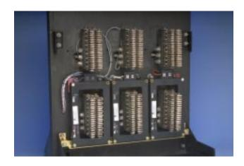
H. Turn the two (2) nylon screws, located in the upper corners of the Sensor Assembly, until they have started in the threaded holes in the Glass Poly Sensor Mounting Plates.
