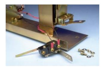
D. Mount the Auxiliary Switch Assembly to the Aux. CT Module Mounting Platform, as shown, using the (2) .164-32 x .500" screws, (4) flat washers, (2) lock washers, and (2) nuts supplied.
