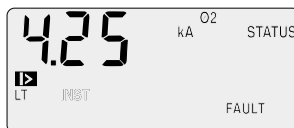
Breaker tripped on long time
