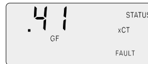
Breaker tripped on ground fault
