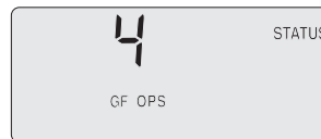
Display showing trip operations counter
