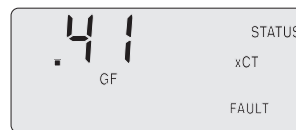
Breaker tripped on ground fault
