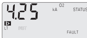
Breaker tripped on long time
