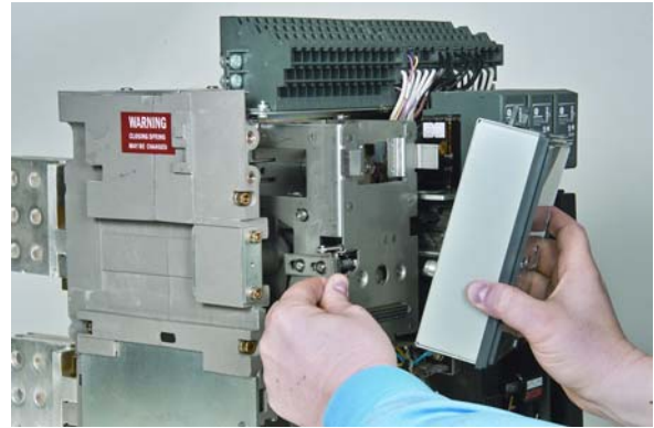
Figure 12. Trip Unit Removal Sequence, Step C
