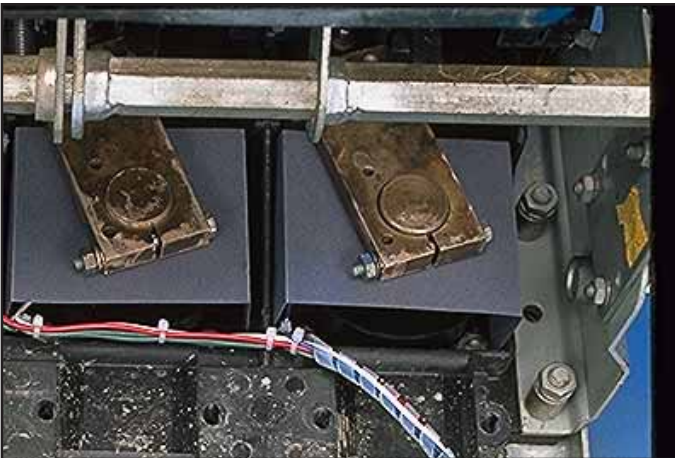
Fig. 4 Shields Installed Over the Sensors.
