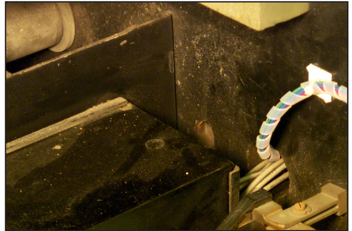
Fig. 10 Sensor Harness Mounted away from the Knife Switch.
