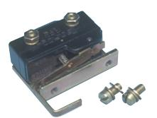
D. Align the Aux. Switch Assembly with the holes in the DTA Assembly. Secure the Aux. Switch Assembly to the DTA Assembly, as shown, using the (2) .190-32 x .375" screws, (2) flat washers, and (2) lock washers provided.
