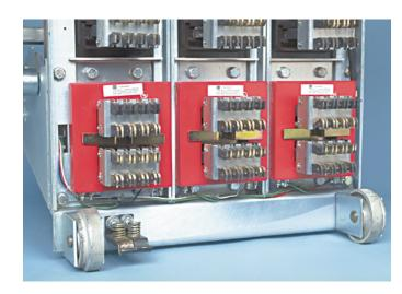
A. Working from the rear of the Breaker, secure each of the (3) Mounting Brackets to the Breaker Back Plate Frames using the (6) .500-13 x 2.50" bolts, (6) lock washers, and (6) flat washers supplied. Note that the Mounting Brackets must be installed with the "risers" facing outwards.
