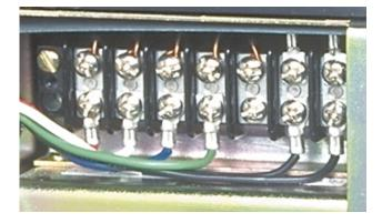
E. Route the Sensor Harness along the front of the Aux. CT Module and then down through the round grommet installed in the Breaker Platform. Route the green wire (with ring terminal) down to the DTA Assembly.
