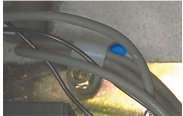
J. Route the HV Wires through Self-Adhesive Wire Clamp with the CPT Harness and the PT Wires.
