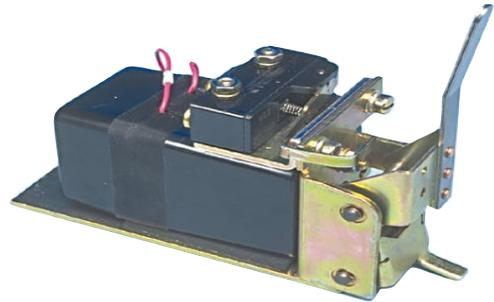
Insure that Aux. Switch moves to the "Closed" position when the DTA Reset Arm is moved towards the DTA.
