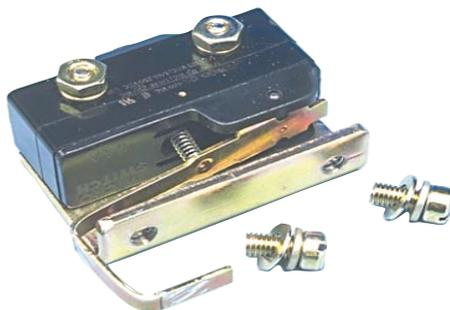
Align the Aux. Switch Assembly with the holes in the DTA Assembly. Secure the Aux. Switch Assembly to the DTA Assembly, as shown, using the (2) .190-32 x .375" screws, (2) flat washers, and (2) lock washers provided.
