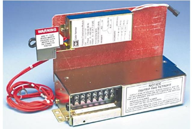
C. Install the Trip Unit on the top of the Aux. CT Module, as shown, using the (2) .190-32 x 4.00" screws, (2) lock washers, and (2) flat washers supplied. Note that the brass spacers are placed between the bottom of the Trip Unit and the top of the Aux. CT Module. Do not completely tighten the screws at this time.
