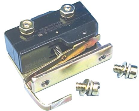
Align the Aux. Switch Assembly with the holes in the DTA Assembly. Secure the Aux. Switch Assembly to the DTA Assembly, as shown, using the (2) .190-32 x .375" screws, (2) flat washers, and (2) lock washers provided.
