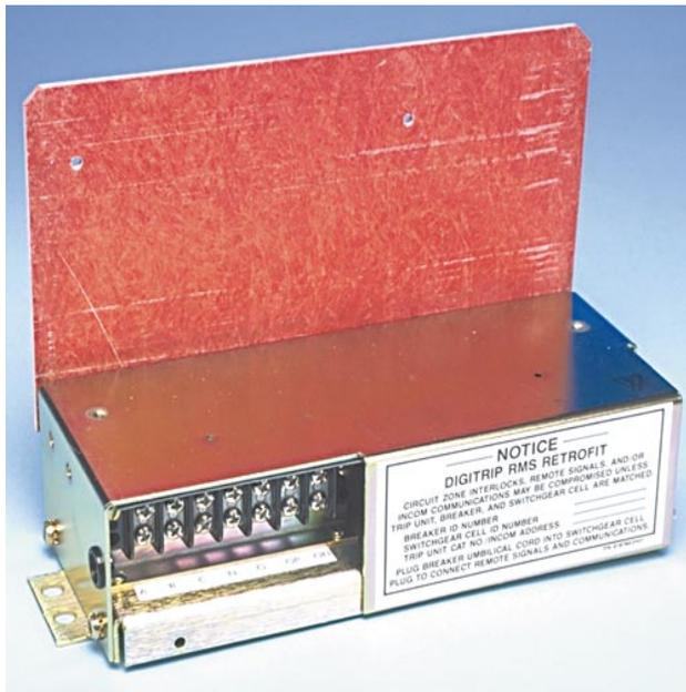
B. For Kits Supplied with a PT Module Only. Mount the PT Module to the Glass Poly Insulation Board, as shown, using the (2) .138-32 x .500" screws, (4) flat washers, (2) lock washers, and (2) nuts supplied.
