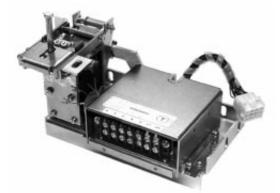
C. Align the holes in the Direct Trip Actuator (DTA) Assembly with the holes in the left front of the Auxiliary (Aux.) CT Module Platform. Using the .164-32 × .312" Pan / Lock screws and flat washers provided, apply Loc-Tite<sup>®</sup> 242 to the threads and mount the DTA Assembly to the Aux. CT Module Platform as shown.
