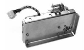
D. Route the DTA Wires over to the Aux. CT Module. Connect the "+" DTA Wire to the "OP" terminal on the Aux. CT Module and the unmarked wire to the "ON" terminal. Fold any excess length of the DTA Wires and secure using the nylon wire tie provided. The excess should then be tucked in between the DTA Assembly and the Aux. CT Module. Make sure that the DTA Wires are clear of any moving parts within the Breaker.
