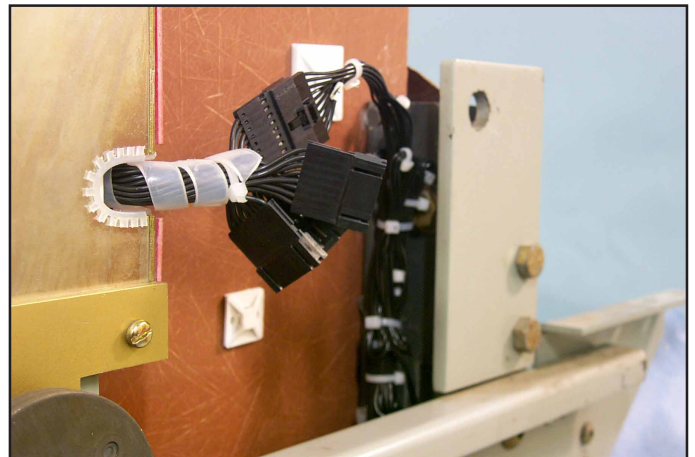
Fig. 43 Routing and Connection of the Aux. CT Harness to the Minibox.
