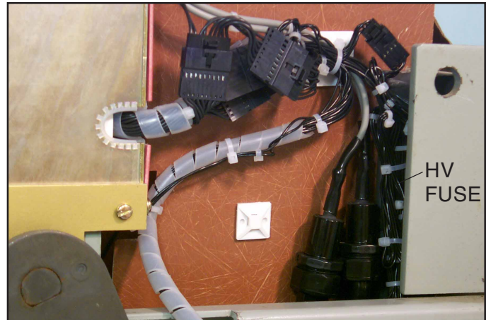
Fig. 57 Suggested Location for the HV Fuses.
