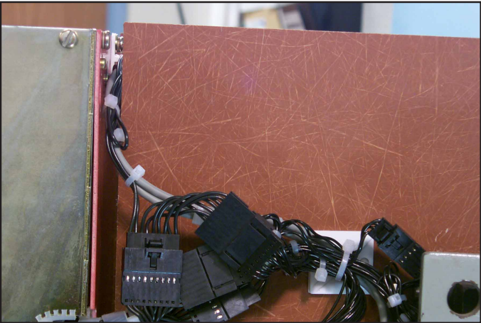
Fig. 55 CPT Harness Connected to the External Harness.
