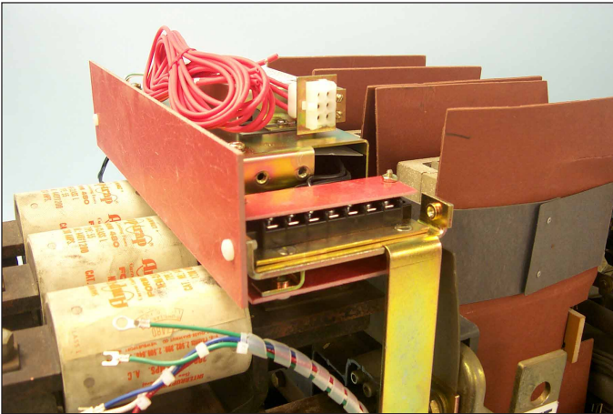
Fig. 20 Rear Aux. CT Module Insulation Barrier Installed on the Mounting Brackets.
