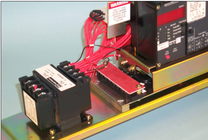
Fig. 17 Connection and Routing of the CPT Wires.
