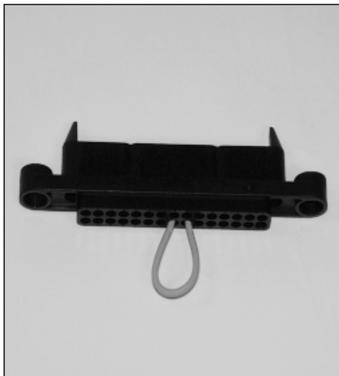
Figure 3. Zone Interlock Shorting Plug
