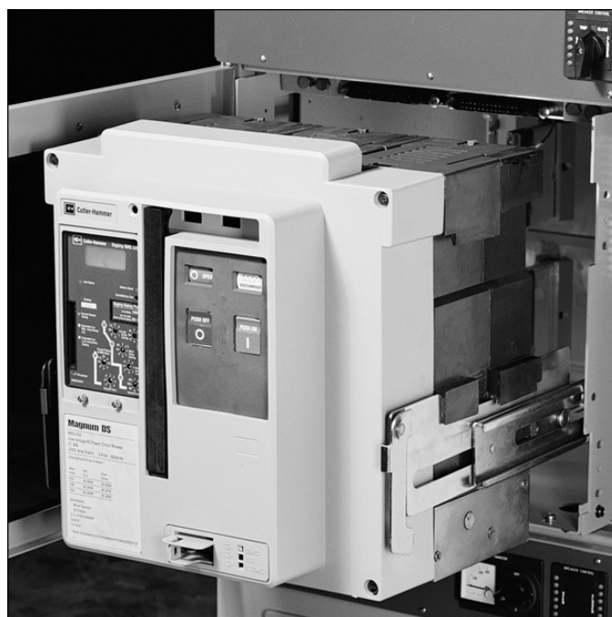
Figure 1-4 Magnum DS Drawout Circuit Breaker Shown on Integral Cassette Extension Rails
