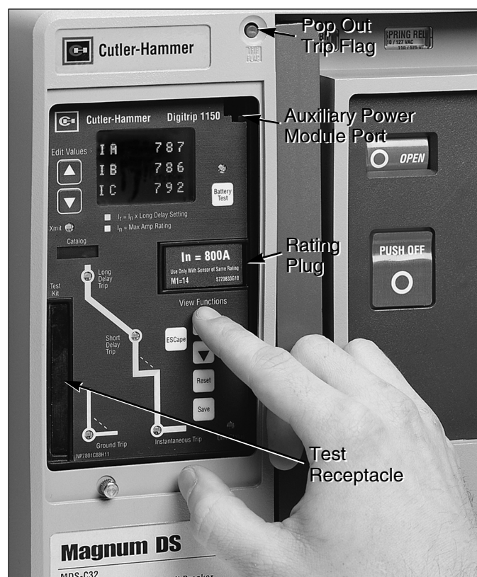
Figure 3-17 Digitrip RMS 1150 Programmable Trip Unit Installed in Magnum DS Circuit Breaker
