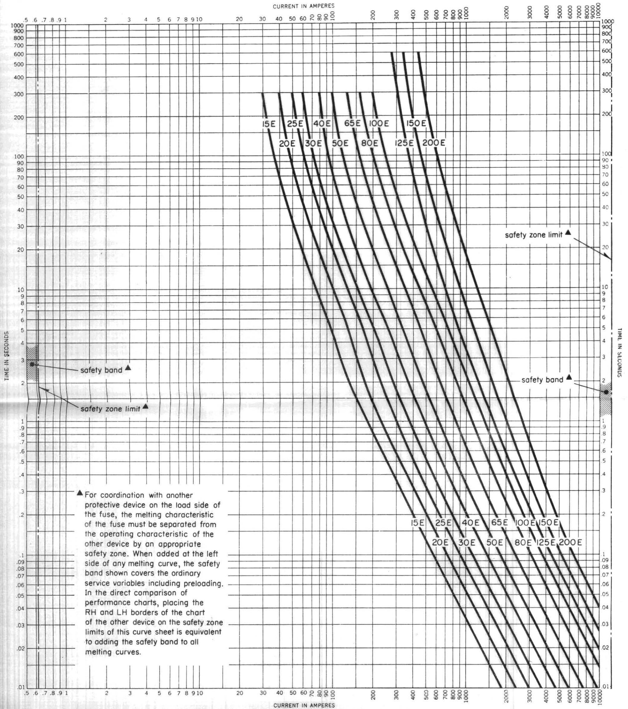
**type DBA-1, -2 and -5 dropout power fuses • time lag fuse elements**
