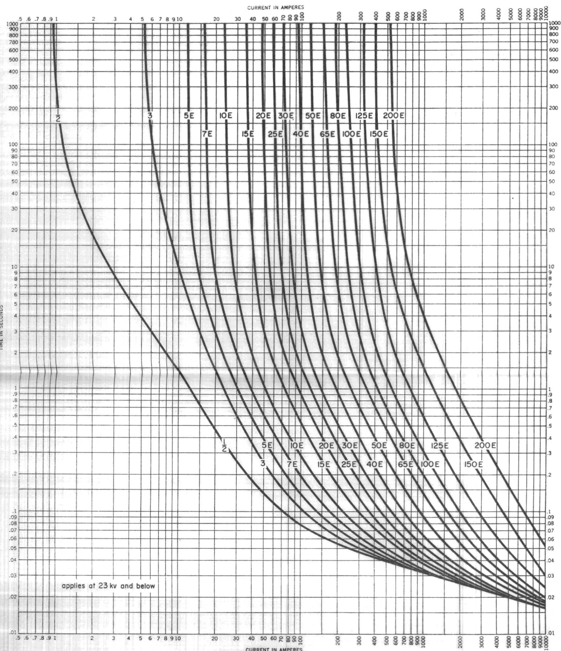
**type DBA-1 dropout power fuses · standard speed fuse elements**
