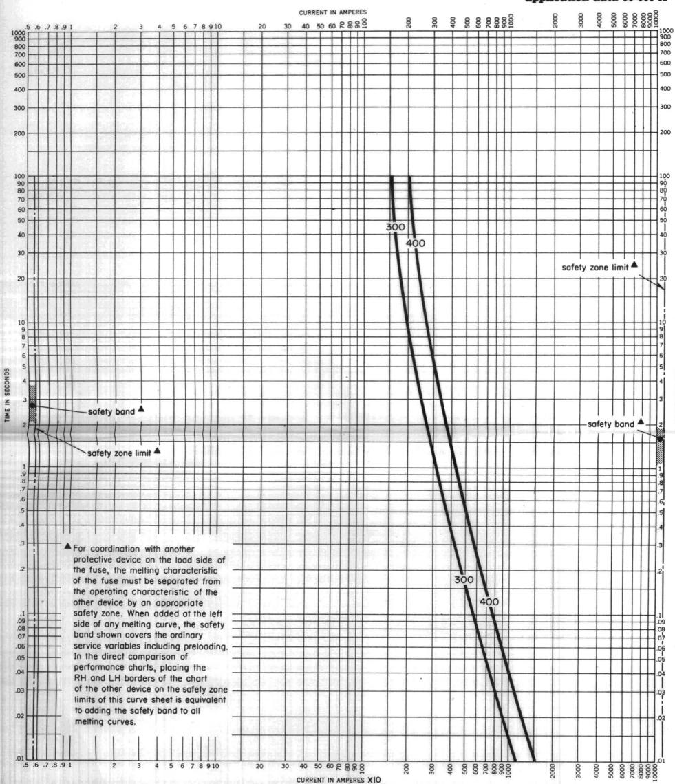
type CLS-2 · current limiting power fuses melting time-current characteristics—2.0 to 5.5 kv
