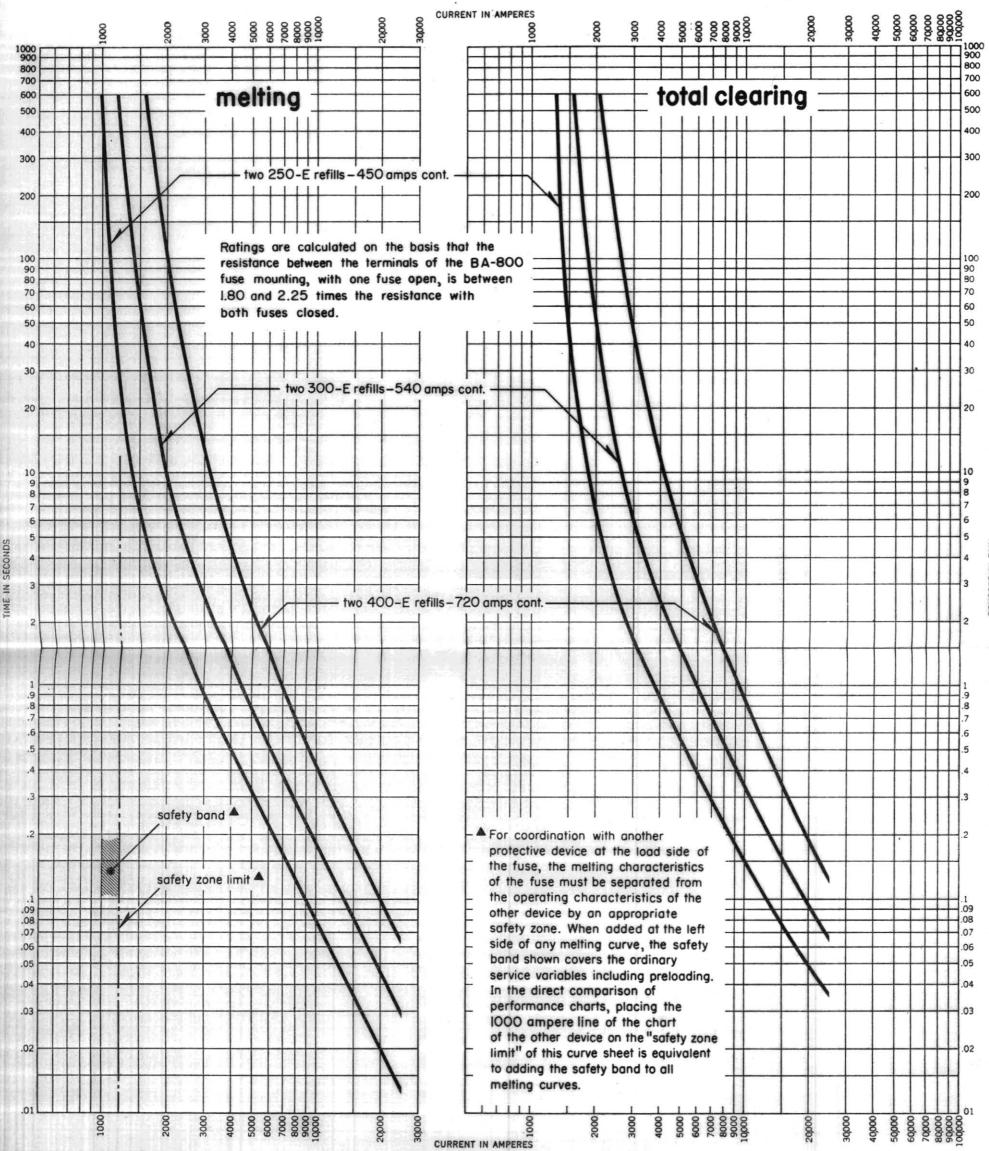
type BA-800 refill power fuse • two BA-400 fuse holders with standard speed refills melting and total clearing time-current characteristics
