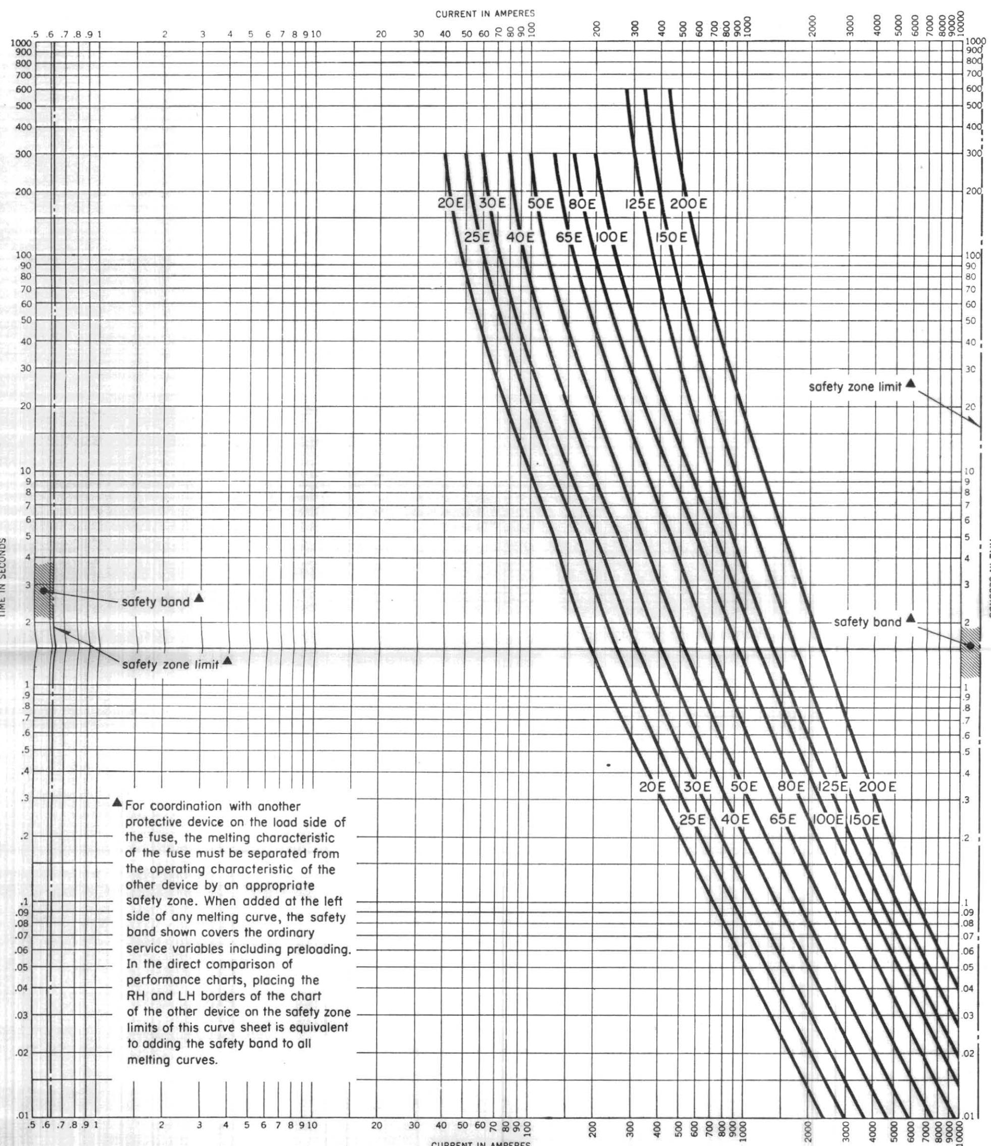
**type BA-400 refill power fuses • time lag refills****melting time-current characteristics**
