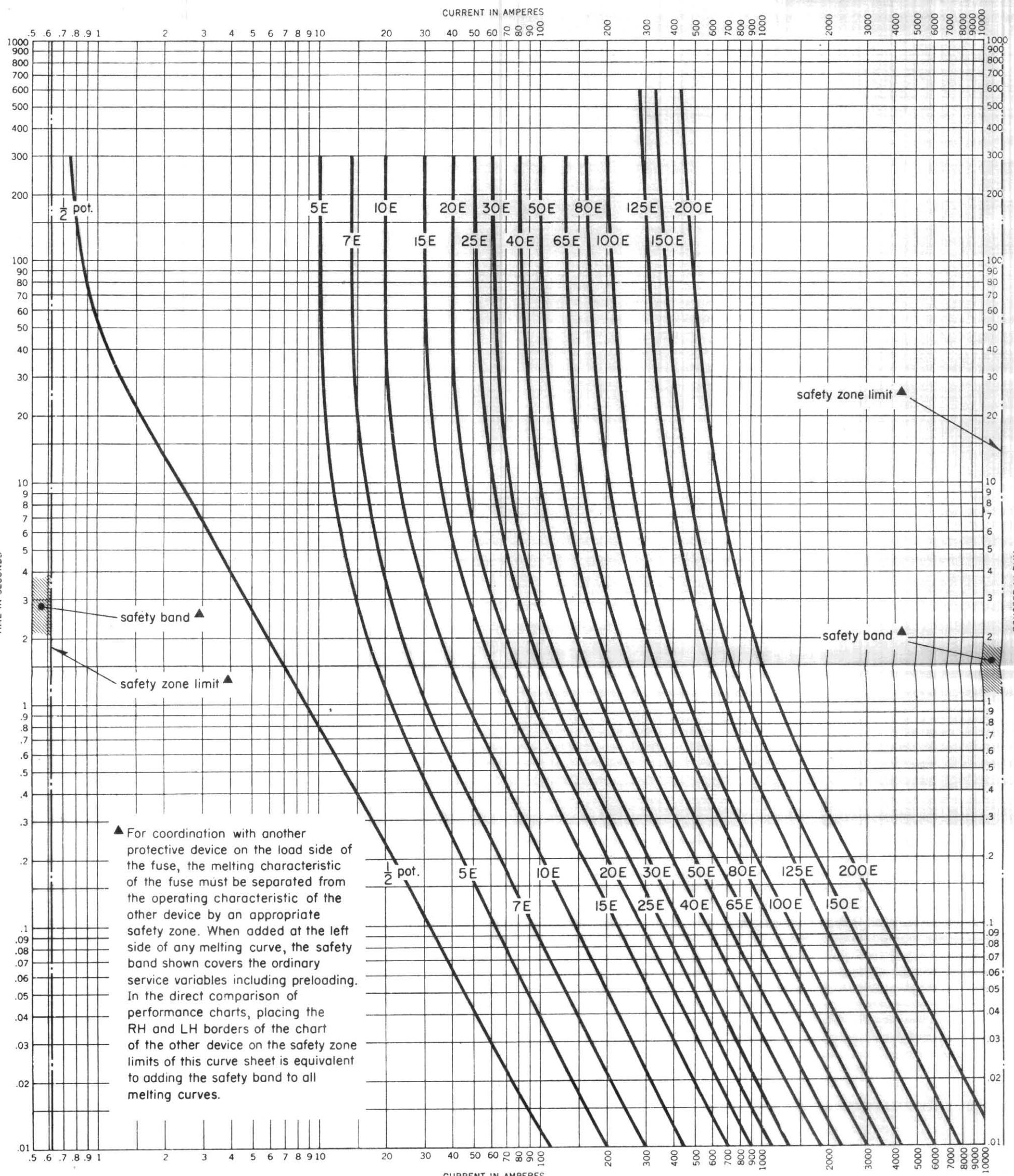
**type BA-200 refill power fuses • standard speed refills****melting time-current characteristics**
