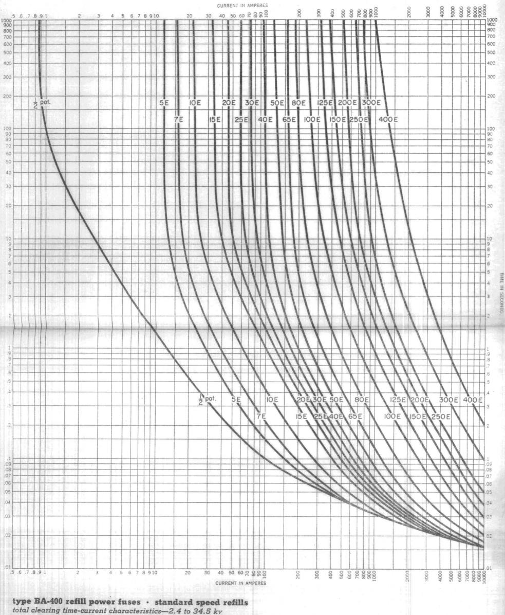
Curves are based on tests starting with fuse unit at an ambient temperature of 25°C and without initial load. Curves are plotted to maximum test points so variations should be negative.
