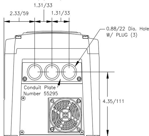
Note: Dimensions are in inches/millimeters
