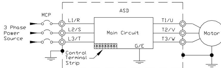
Connect the 3-phase input power to the input terminals of the ASD at **L1/R**, **L2/S**, and **L3/T**. Connect the output of the ASD to the motor from terminals **T1/U**, **T2/V**, and **T3/W**. The input and output conductors and terminal lugs used shall be in accordance with the requirements listed in Cable/Terminal Specifications on pg. 57.
