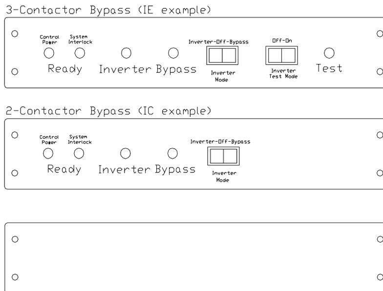
**Control Power LED (LED 5)** — On when the control circuit power is available. This is not an indication that power is off.
