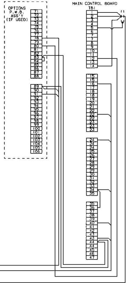
LOW LEVEL CONTROL WIRING. THESE CONDUCTORS MAY BE ROUTED IN THE SAME RACEWAY. MAINTAIN 3" SEPARATION (CONDUIT) OR 12" SEPARATION (TRAY) FROM OTHER TYPES OF POWER OR CONTROL WIRING. ALL CONDUCTORS TO BE #18 AWG MINIMUM. SHIELDED CABLE TO BE JACKETED. GROUND SHIELD ONLY WHERE SHOWN. INSULATE OTHER END OF SHIELDED CABLE.
