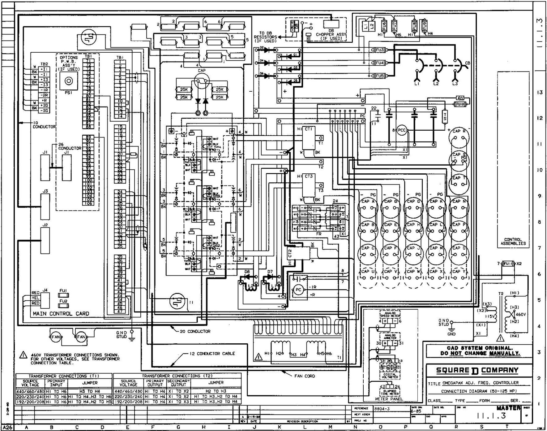
⚠ 460V TRANSFORMER CONNECTIONS SHOWN. FOR OTHER VOLTAGES, SEE TRANSFORMER CONNECTION TABLE.
