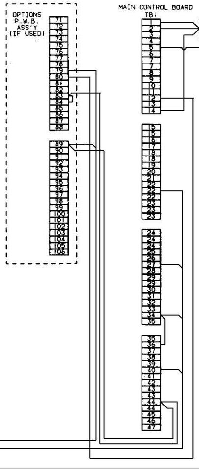
LOW LEVEL CONTROL WIRING. THESE CONDUCTORS MAY BE ROUTED IN THE SAME RACEWAY. MAINTAIN 3" SEPARATION (CONDUIT) OR 12" SEPARATION (TRAY) FROM OTHER TYPES OF POWER OR CONTROL WIRING. ALL CONDUCTORS TO BE #18 AWG MINIMUM. SHIELDED CABLE TO BE JACKETED. GROUND SHIELD ONLY WHERE SHOWN. INSULATE OTHER END OF SHIELDED CABLE.
