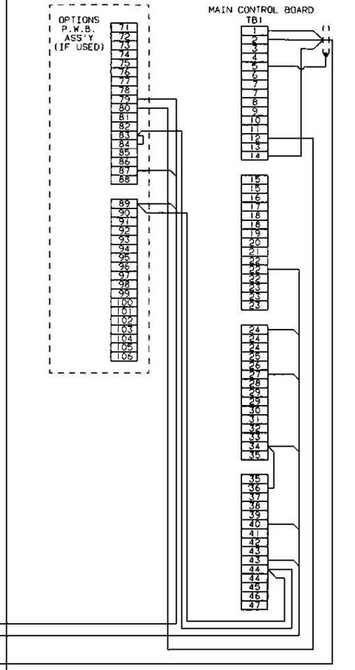
LOW LEVEL CONTROL WIRING. THESE CONDUCTORS MAY BE ROUTED IN THE SAME RACEWAY. MAINTAIN 3" SEPARATION (CONDUIT) OR 12" SEPARATION (TRAY) FROM OTHER TYPES OF POWER OR CONTROL WIRING. ALL CONDUCTORS TO BE #18 AWG MINIMUM. SHIELDED CABLE TO BE JACKETED. GROUND SHIELD ONLY WHERE SHOWN. INSULATE OTHER END OF SHIELDED CABLE.
