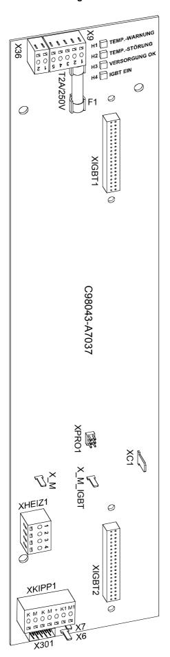
X36 Internal connector Overtemperature alarm relay
