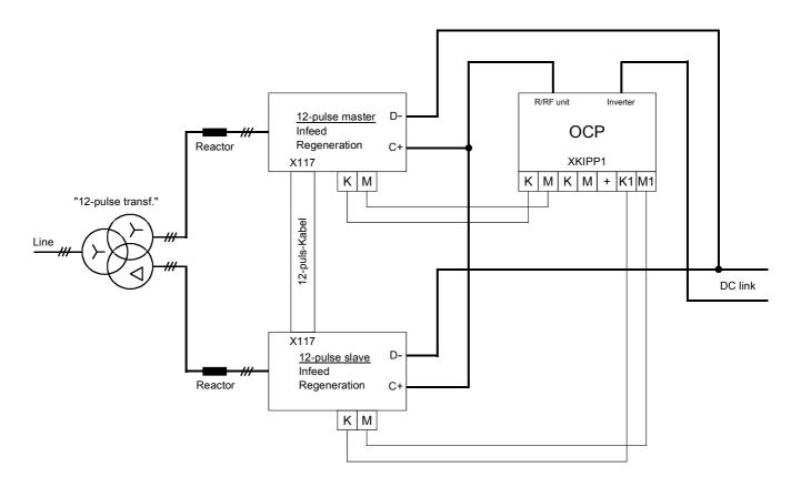
Redundant operation is no longer an option since the failed R/RF unit shuts down the OCP via terminals K and M.
