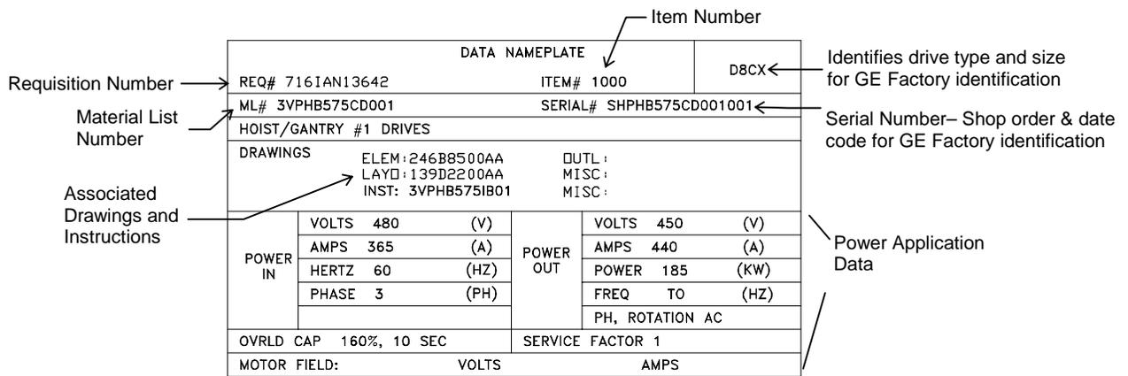
Figure A-4. Typical Drive Nameplate
