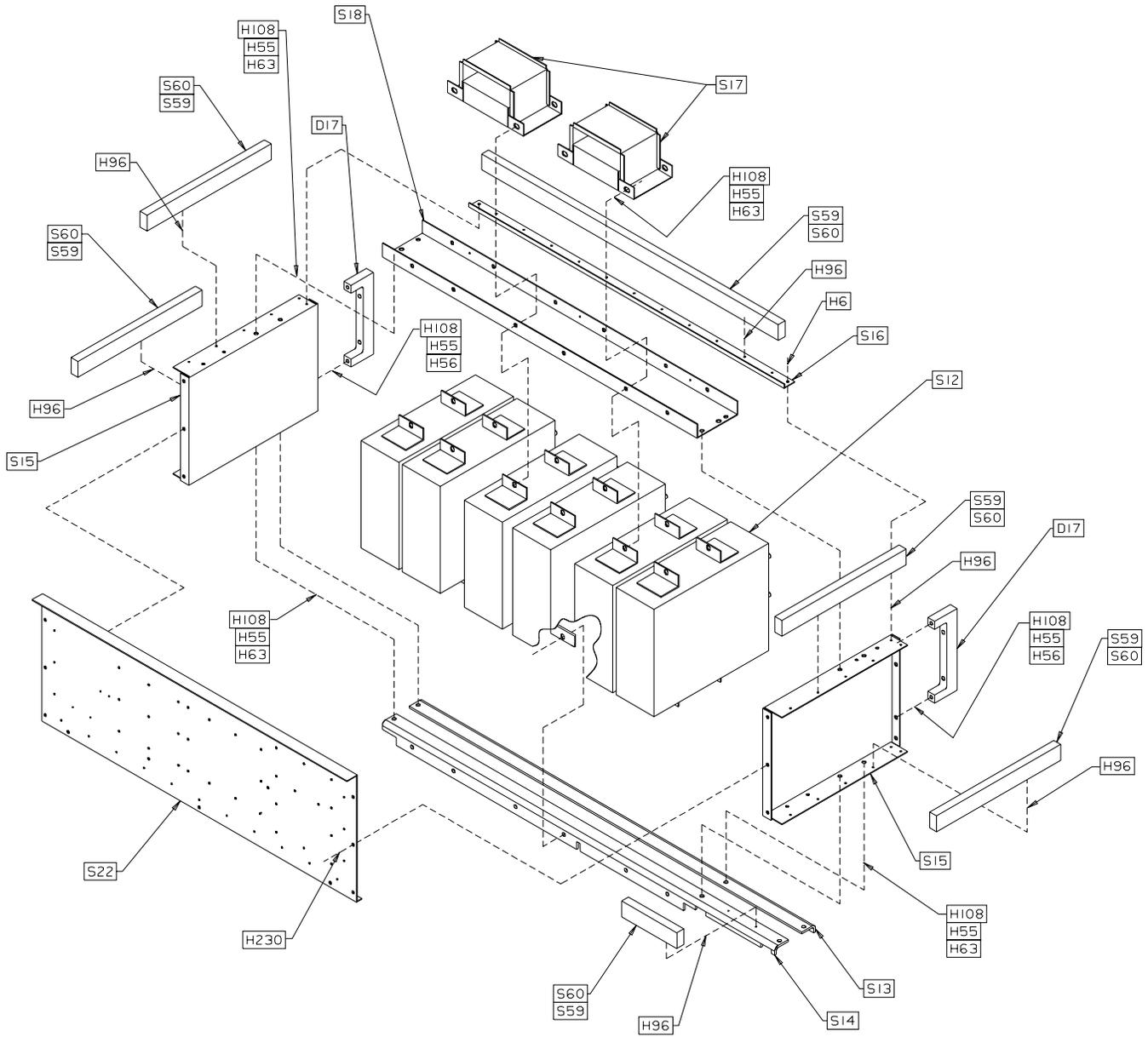
Figure C-1. DC Link Capacitor Assembly
