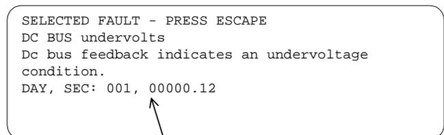
Figure 2-12. Sample Fault Detail Screen
