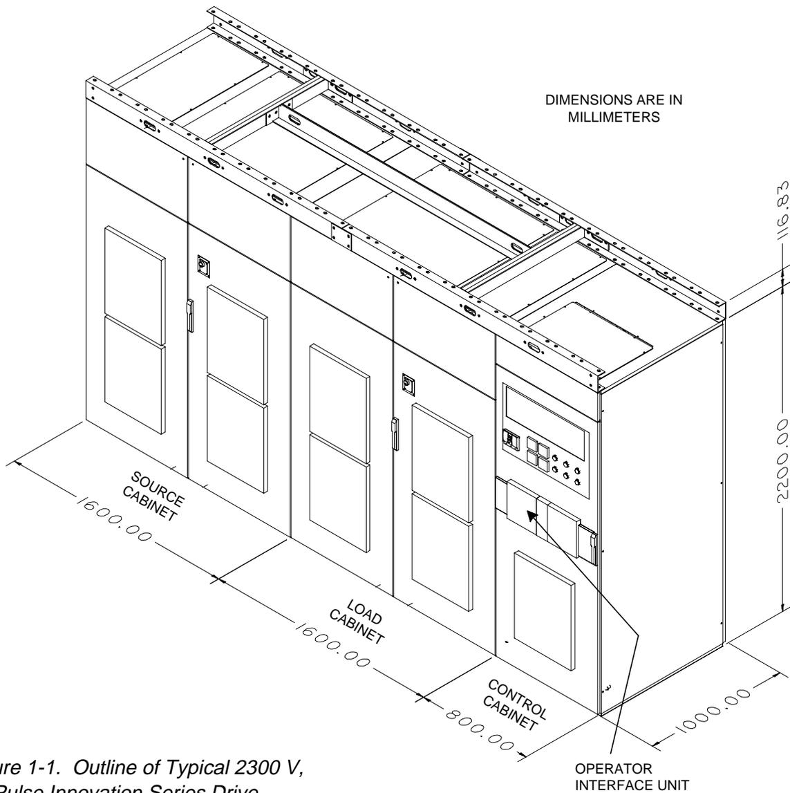
Figure 1-1. Outline of Typical 2300 V, 18-Pulse Innovation Series Drive
