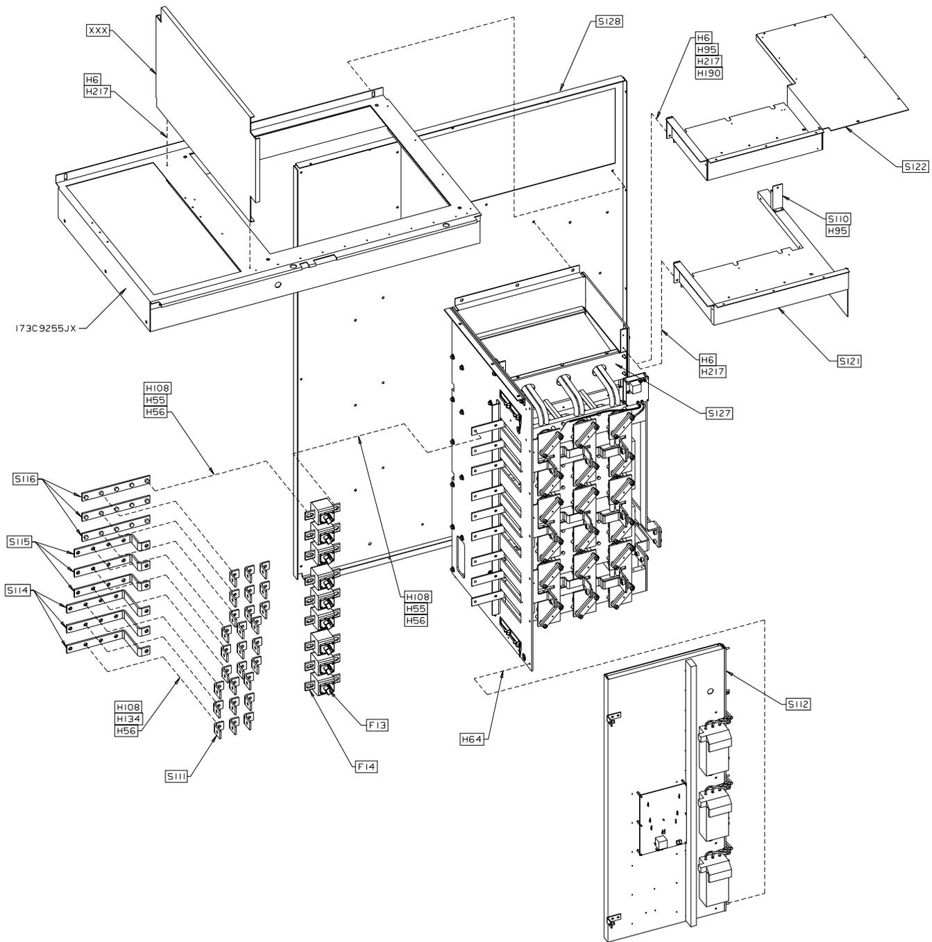
Figure C-9. Panel Assembly, Source Cabinet
