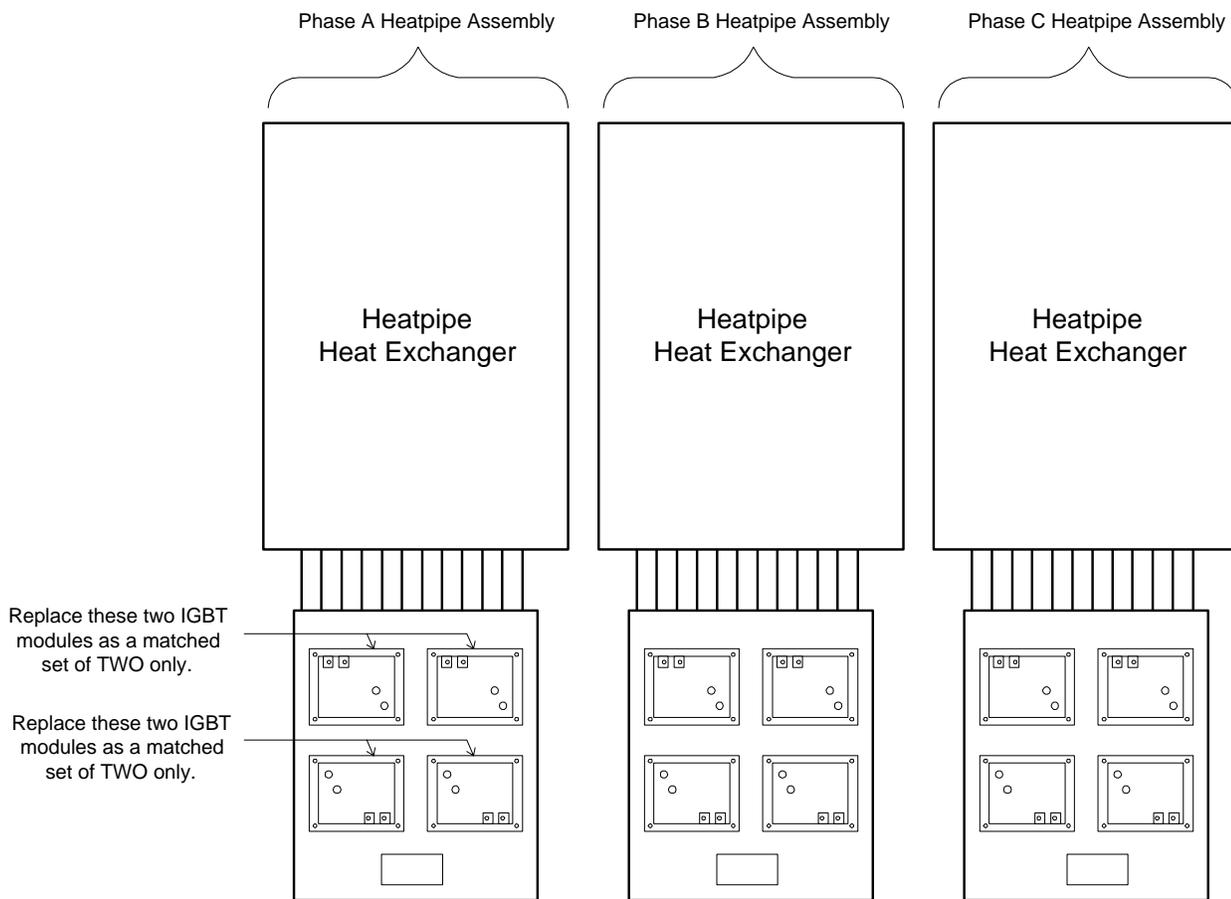
Figure 5-1. IGBT Module Location in 2300 V Drive Heat Exchanger Assembly
