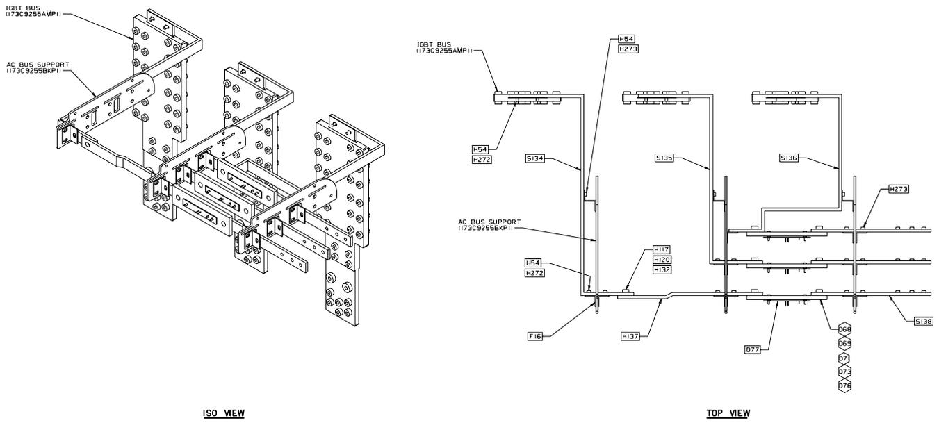
Figure C-3. Back Panel Assembly Showing IGBT Bus, Load Cabinet
