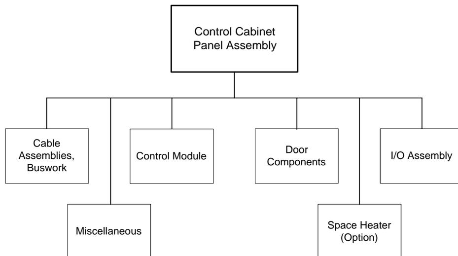
Figure 6-3. Parts List Structure, Control Cabinet
