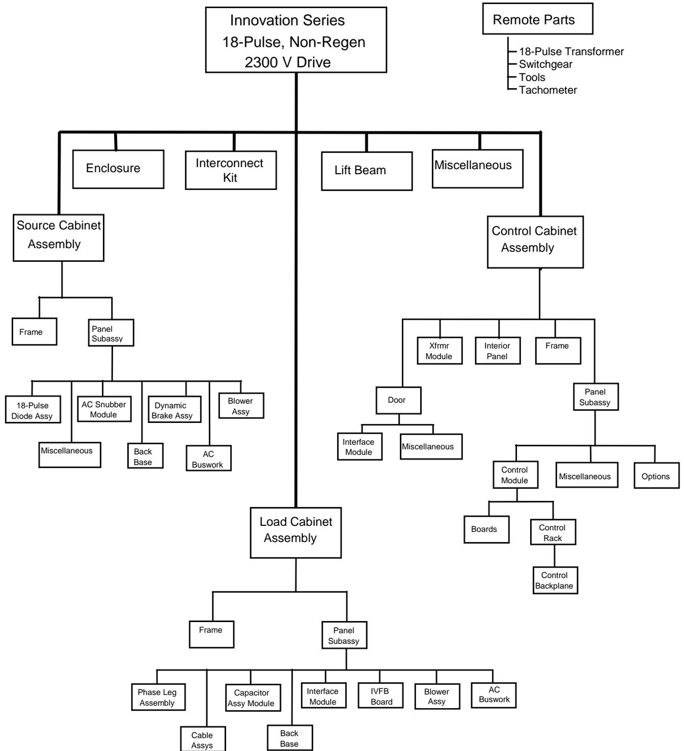
Figure 1-2. Overview of Drive Hardware Structure
