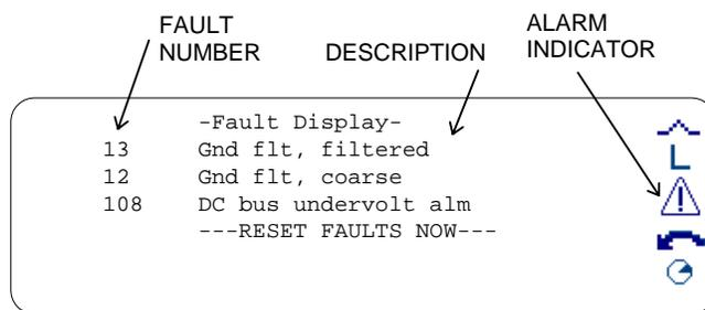
Figure 4-1. Example of DDI Fault Display Screen
