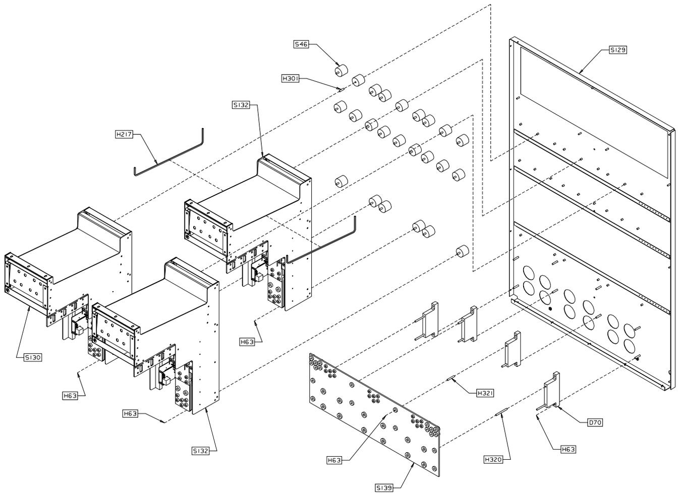
Figure C-2. Back Panel Assembly, Load Cabinet
