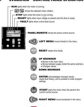
STOP stops the motor when the panel is the
