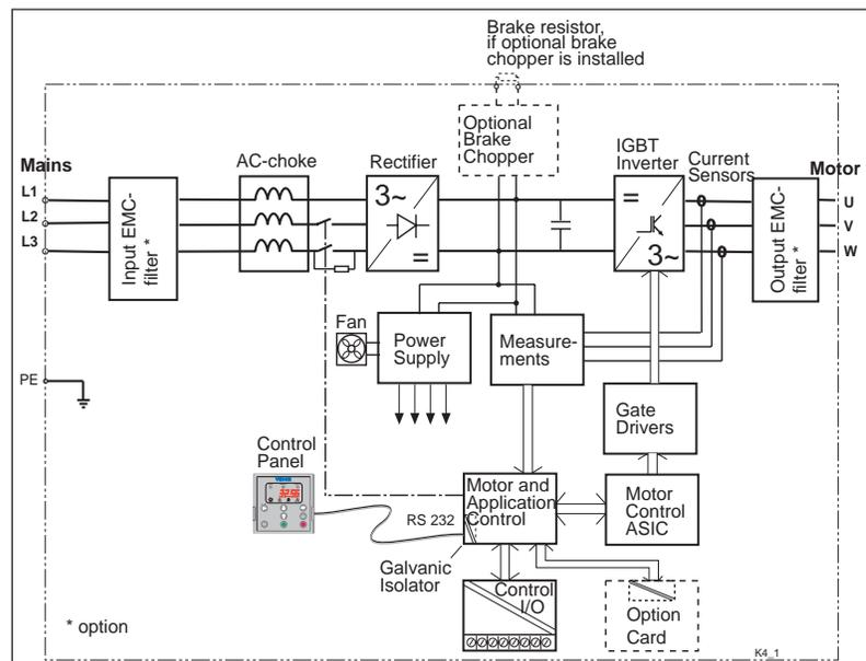
Figure 4-1 SV9000 block diagram.
