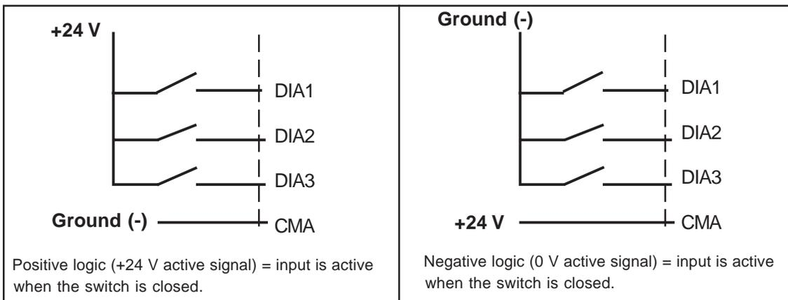
Figure 6.2.3-1 Positive/negative logic.
