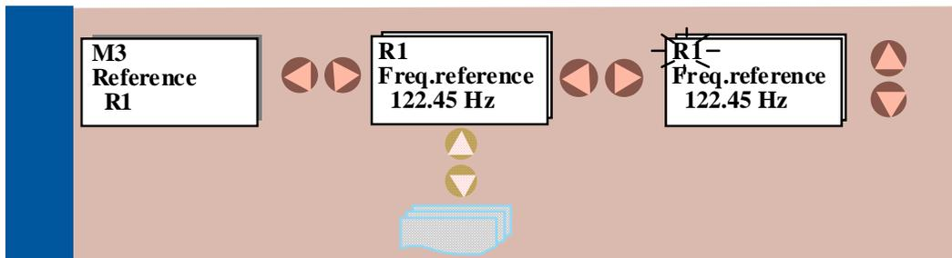
*Figure 7.5-1 Reference setting on the control panel*
