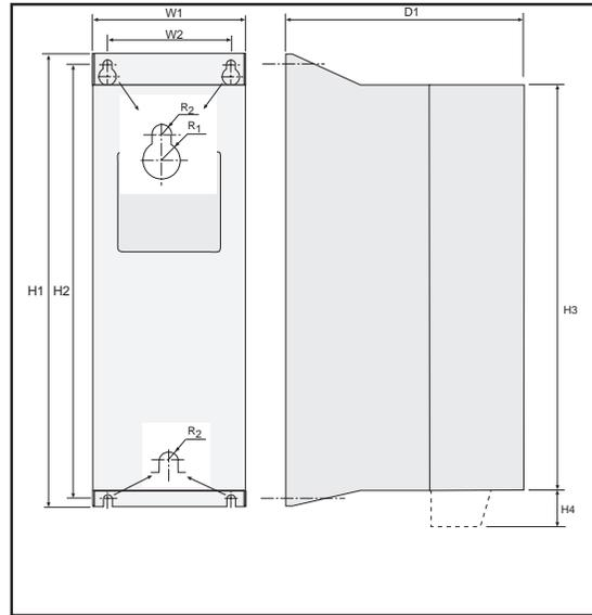
Figure 5.3-1 Mounting dimensions.
